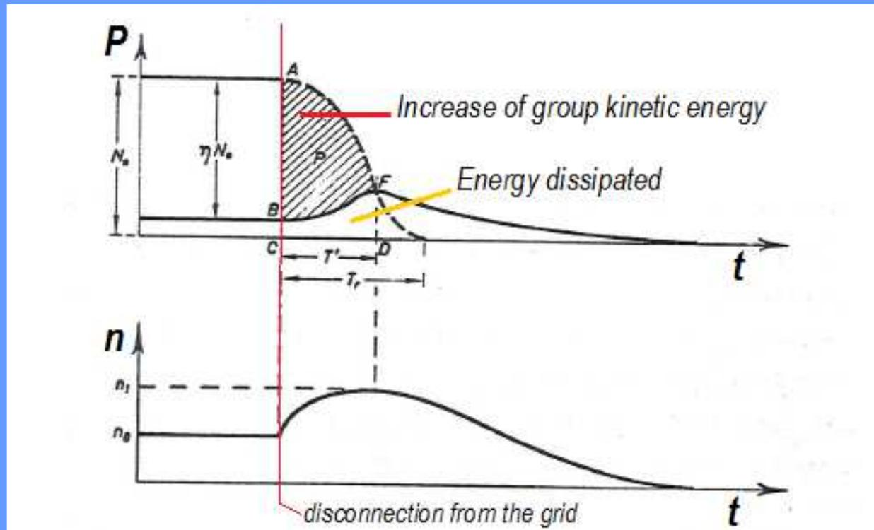
Time evolution of Power delivered ( $P$ ) on the turbine axis and rotational speed ( $n$ ) as a function of a sudden disconnection from the grid
