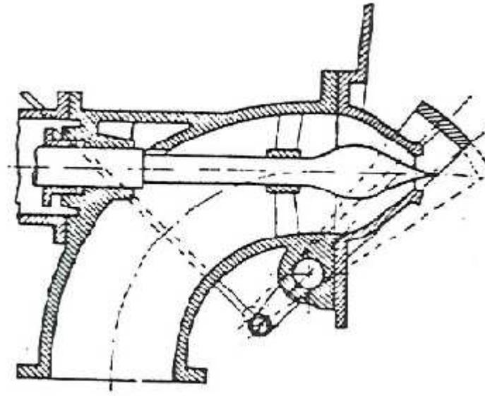
In a Pelton turbine the discharge is controlled through a needle valve (spina di regolazione o ago dabile) and sudden shut down are operated through a deflector (tegolo deviatore)
