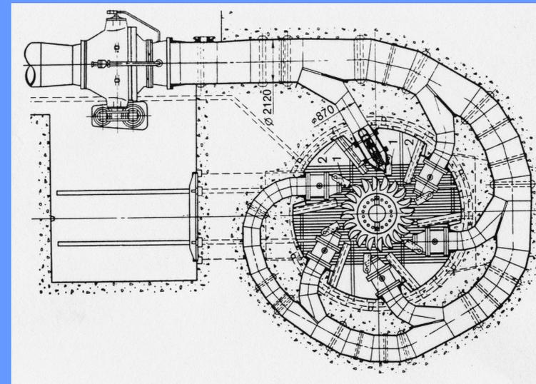
CIMEGO Plant (110 MW, H 721 m, D=3.5m, n= 300rpm, d 0.31 m)
