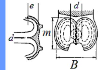
2) The dimension  $B$  of the bucket and  $D$  of the runner are obtained by empirical rules of thumb as in the diagrams below
