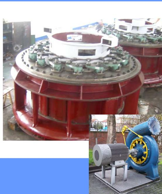
In a Francis turbine the discharge is controlled by the distributor, that is formed by a certain number of mobile blades, whose group constitutes a concentric ring around the impeller. Its function is to distribute, regulate or cut totally, the water flow that flows toward the impeller.
