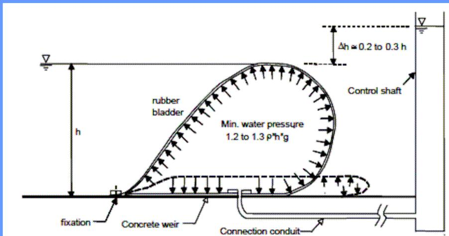
*Inflatable weir: a simple and economic proxy, particularly when the water raise is limited and the span considerable.*
