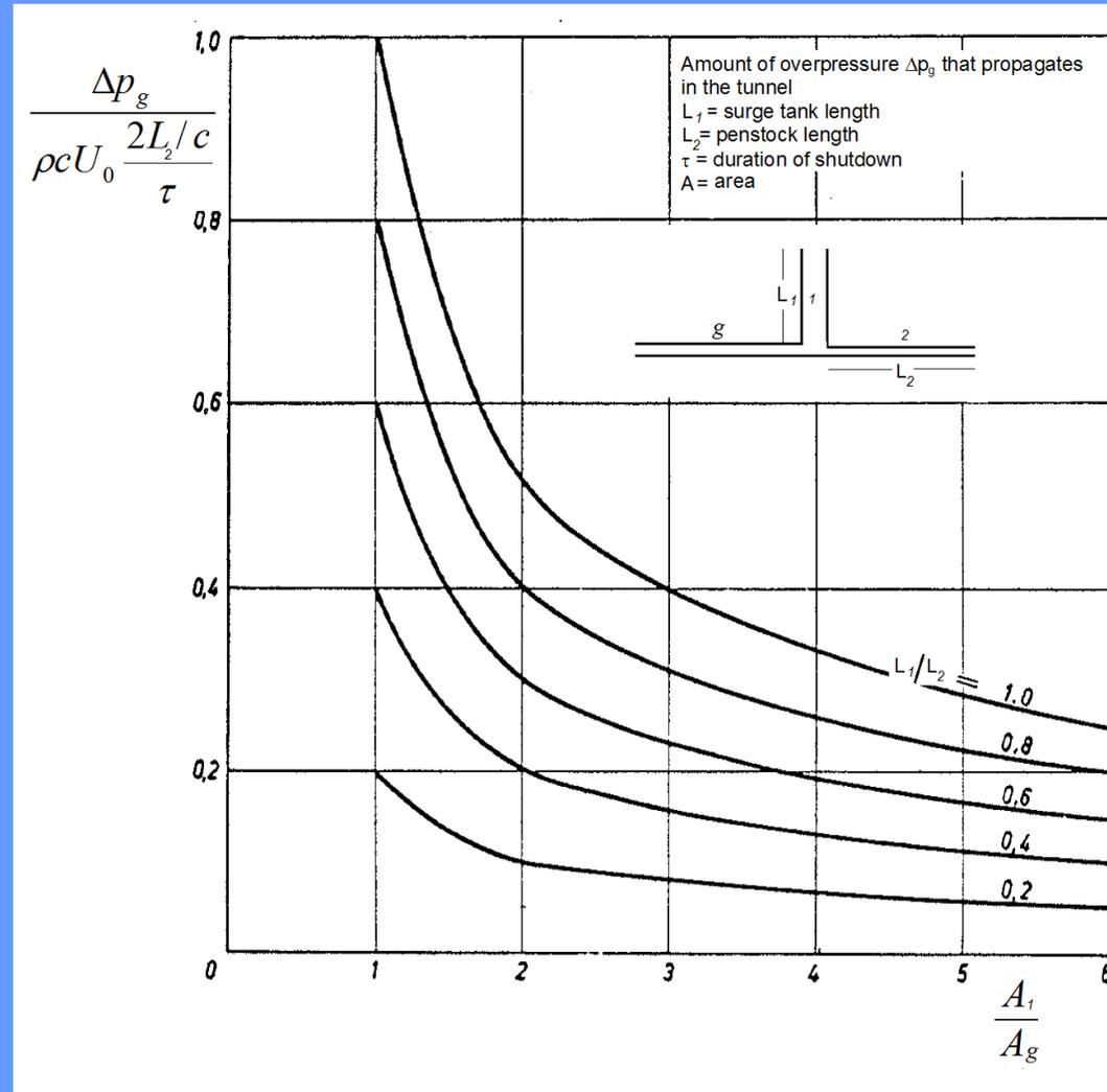
This theoretical graph shows the strong overpressure reduction in the tunnel even when the surge tank cross section area is slightly larger than the cross section area of the penstock
