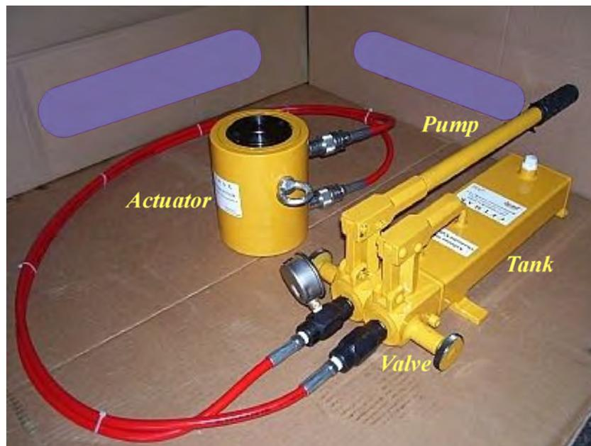
Figure 6.4: *Hydraulic double-acting cylinder with manual pump (Courtesy of RITM industry)*
