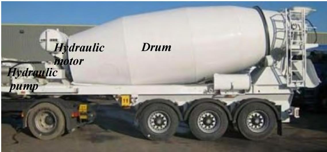
Figure 1.5: *Concrete mixer (Courtesy of Liebherr)*
