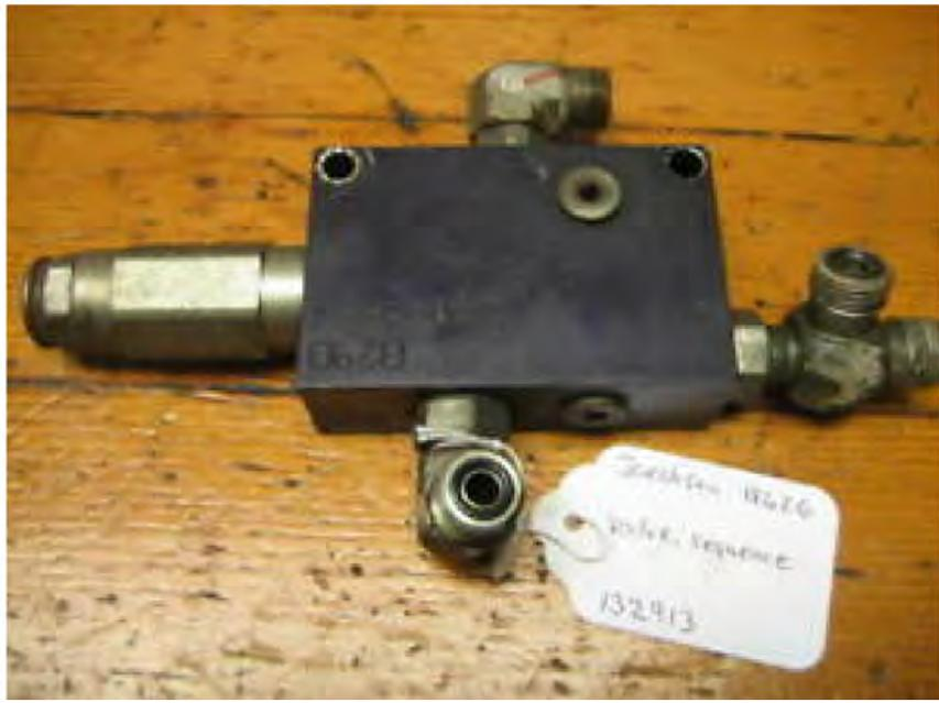
Figure 8.28: Sequence valve (Courtesy of JACOBSEN)
