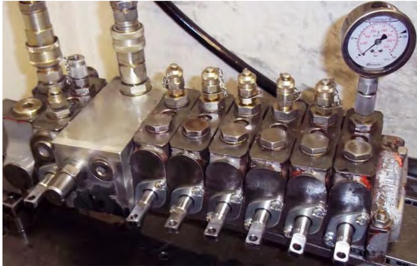
Figure 8.31: *Modular valves (Courtesy of Hydrastar)*
