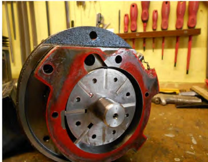
Figure 8.13: *Vane Compressor (Courtesy of Linqvip)*
