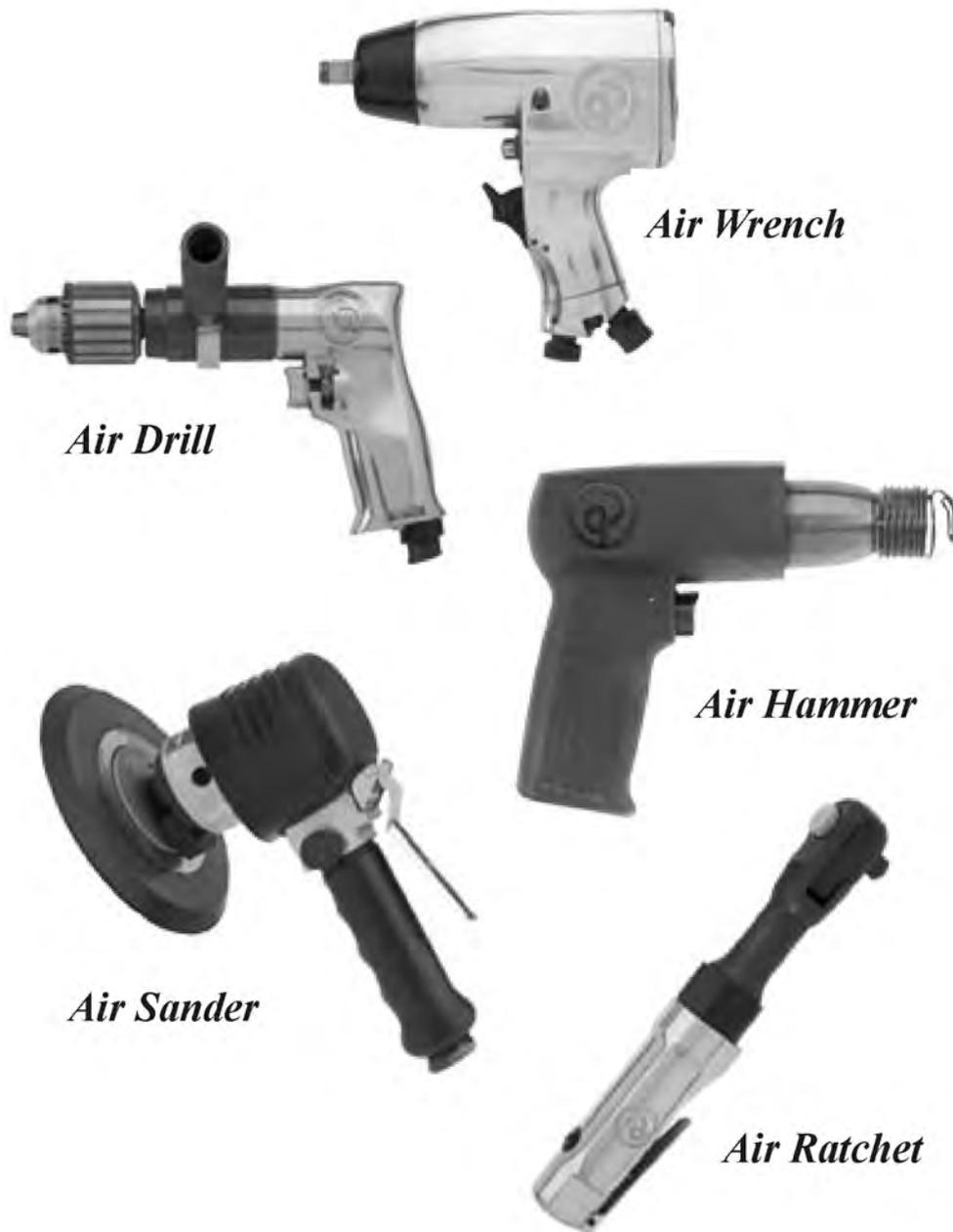
Figure 1.13: *Different pneumatic tools (courtesy of Industrial Hardware)*
