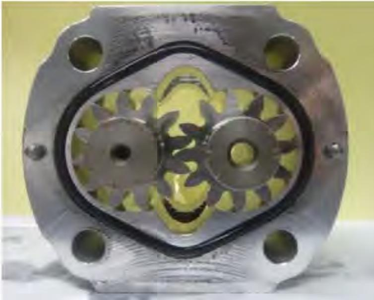
Figure 8.20: Gear motor
