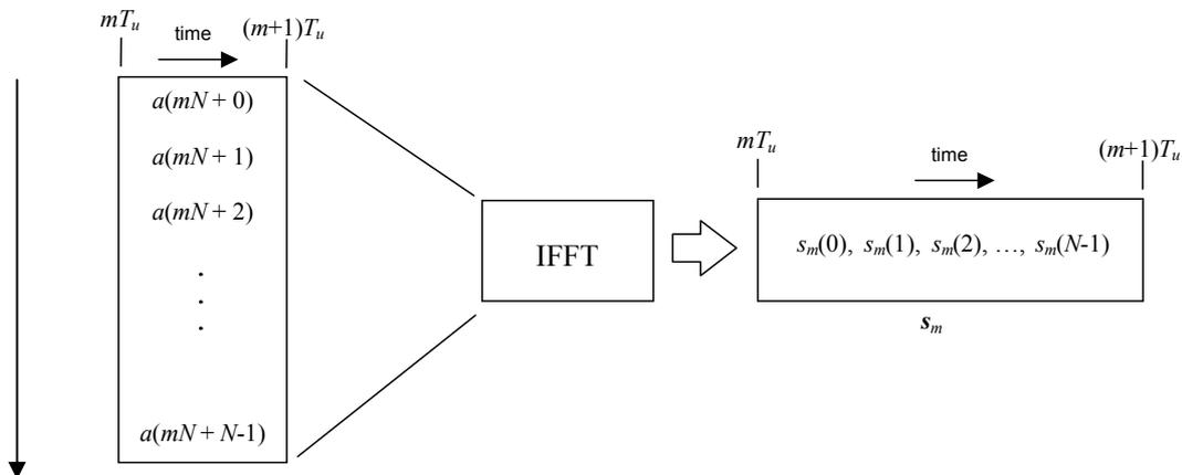
**Figure 3: OFDM useful symbol generation using an IFFT [Ref. 2]**
