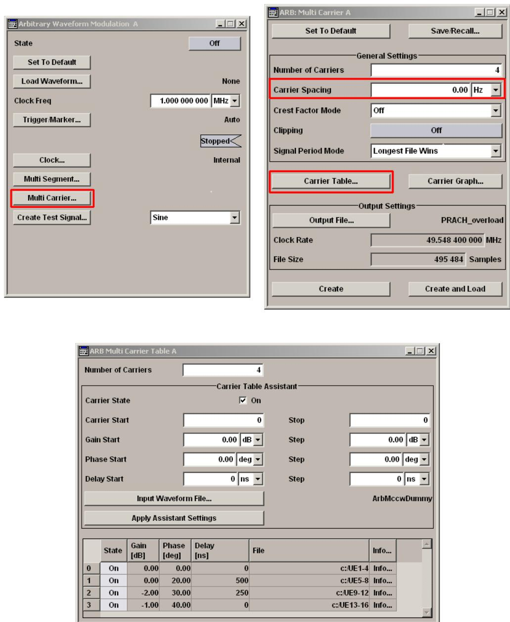
Figure 52: Creating a Multi-carrier ARB file for LTE PRACH overload testing
