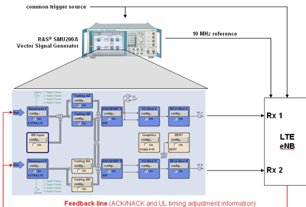
Figure 48: Measurement setup for UL timing adjustment acc. to section 8.2.2. in TS 36.141 [Ref.16]
