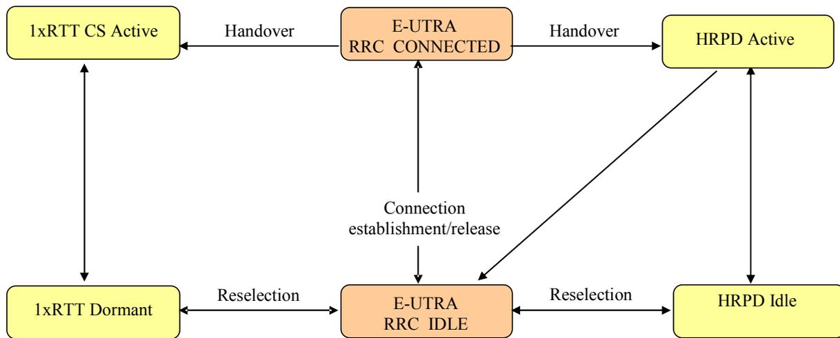
**Figure 33: Mobility procedures between E-UTRA and CDMA2000 [Ref. 9], HRPD = High Rate Packet Data**
