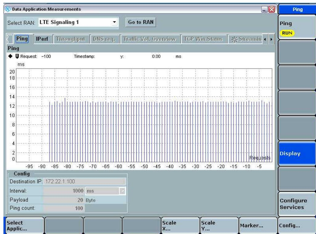
**Figure 1: PING test (about 12 ms) using Data Application Unit (DAU) in R&S® CMW500 Wideband Radio Communication Tester while doing data end-to-end (E2E) testing for UMTS LTE (FDD)**
