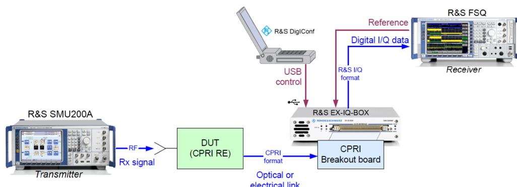
Figure 57: Test setup for RE testing (Uplink)
