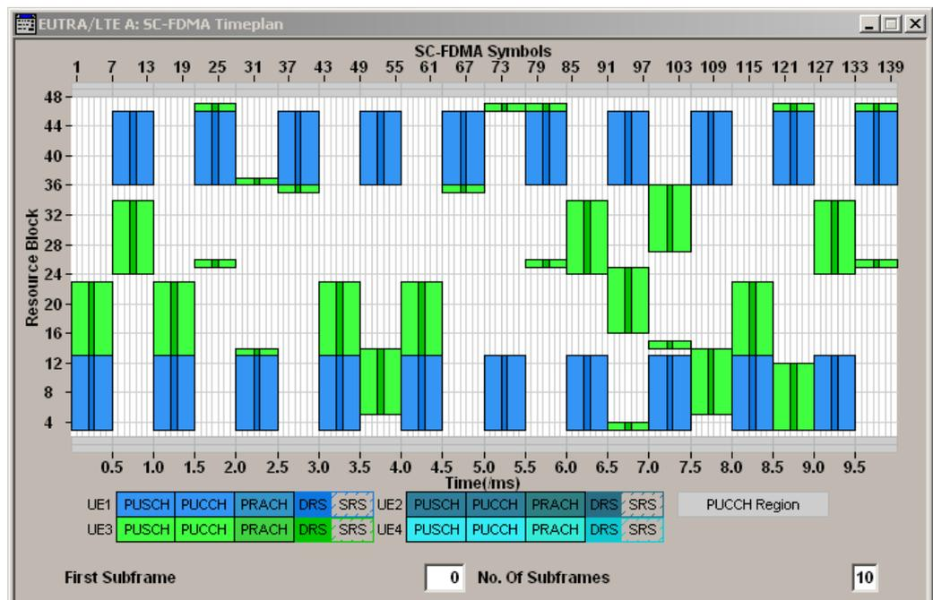
Figure 19: Intra-subframe hopping, Type 1 (blue, UE1) and Type 2 (green, UE3)
