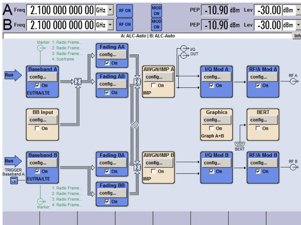
**Figure 67: User interface of the SMU200A signal generator for 2x2 MIMO tests: The signal flow is shown from the generation of the two baseband LTE signals on the left via the four fading channels to the two RF outputs on the right.**
