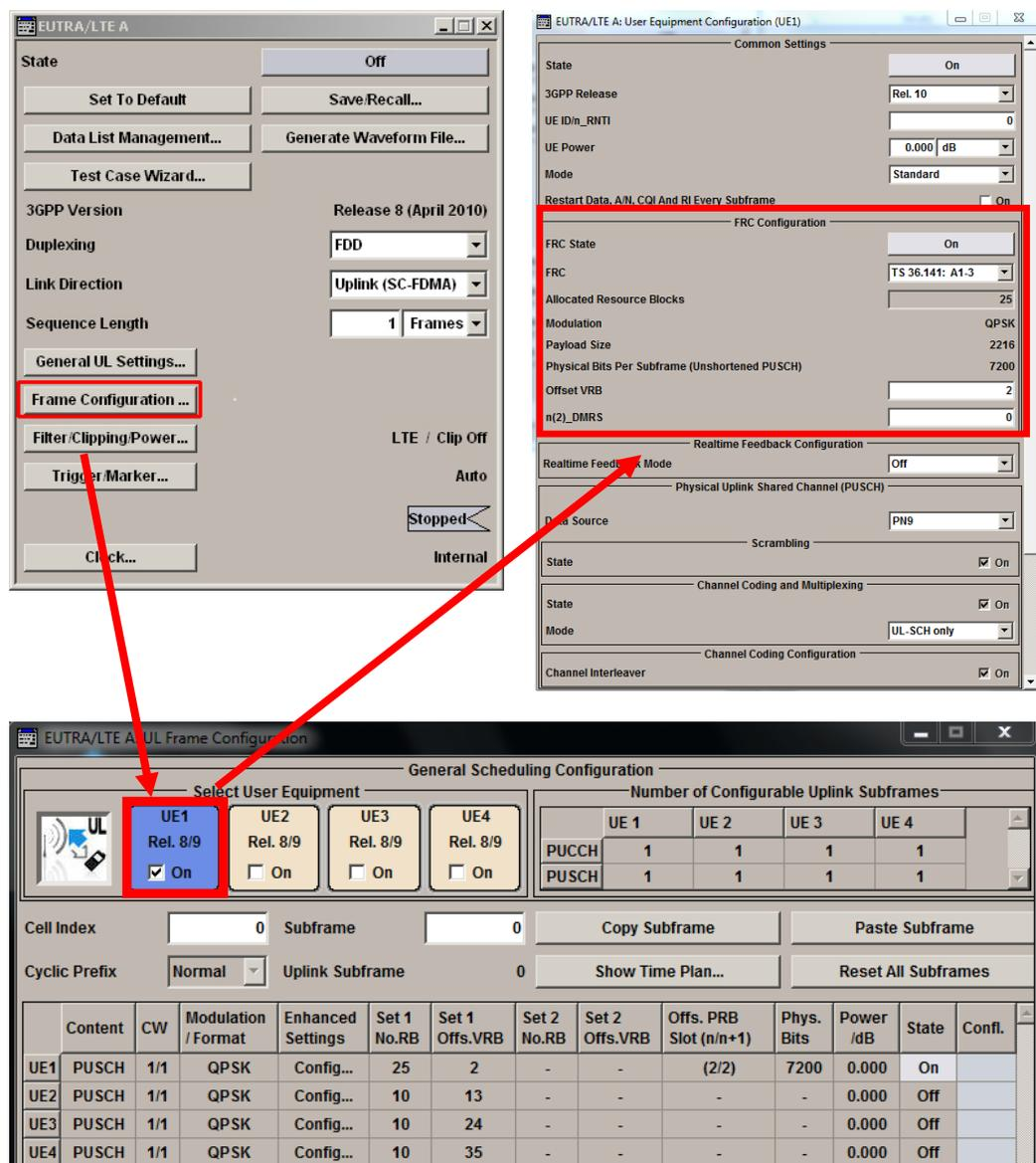
Figure 46: Configuring FRC on R&S@SMU200A Vector Signal Generator
