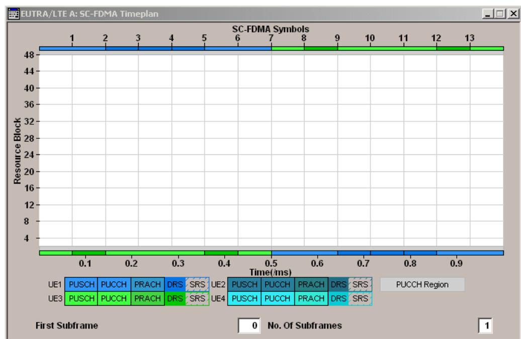
**Figure 20: Example for PUCCH resource allocation (UE1: format 1a, UE3: format 2)**
