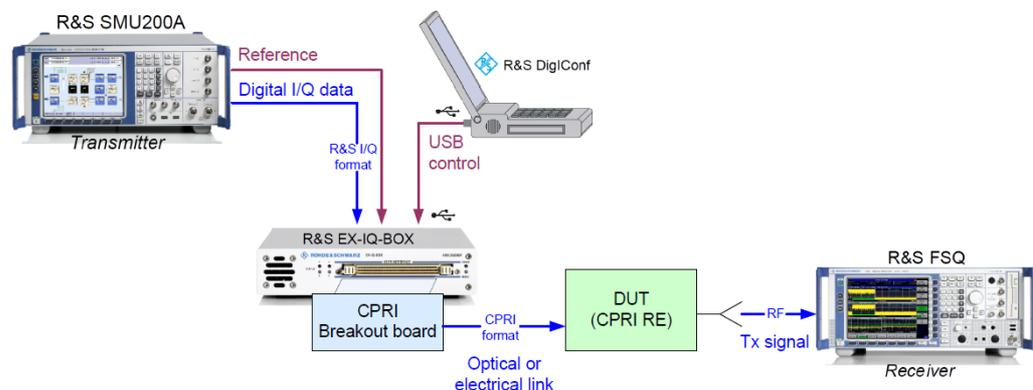
Figure 56: Test setup for RE testing (Downlink)
