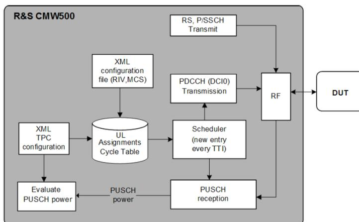
**Figure 65: Block diagram for testing PUSCH power control (uplink), R&S®CMW-KF506**
