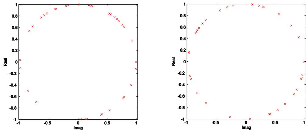
**Figure 21: Uplink reference signal sequences for an allocation of three resource blocks, generated by different cyclic shifts of the same base sequence**
