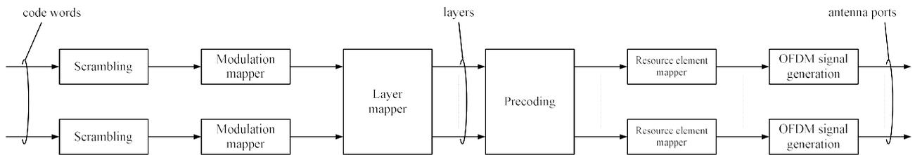
**Figure 26: Overview of downlink baseband signal generation [Ref. 3]**
