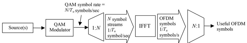
**Figure 4: OFDM Signal Generation Chain [Ref. 2]**
