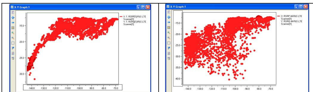
Figure 83: RSRP (x-axis) versus RSRQ (y-axis) comparison, indicating no pilot pollution (left) and pilot pollution (right)
