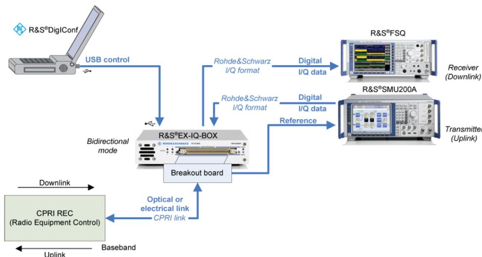
Figure 58: Test setup Radio Equipment Controller (REC) testing with R&S EX-IQ-BOX
