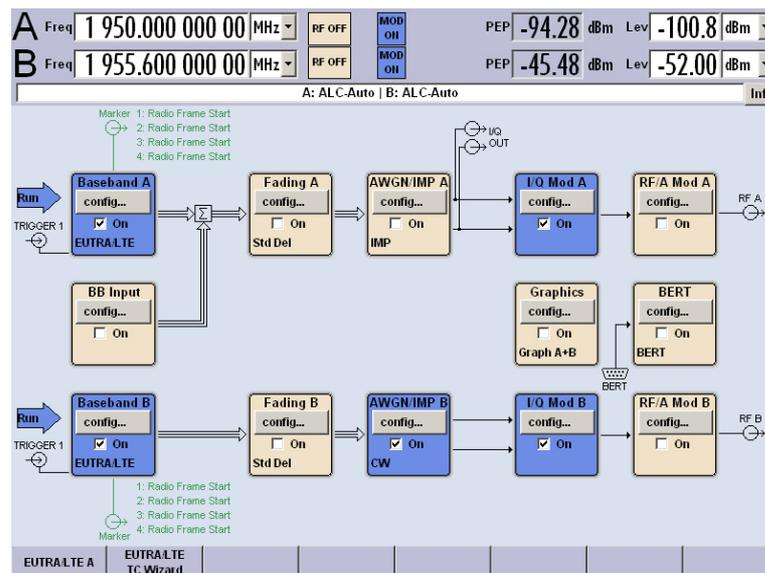
Figure 50: SMU200A block diagram for receiver intermodulation acc. to TS 36.141 [Ref. 16]
