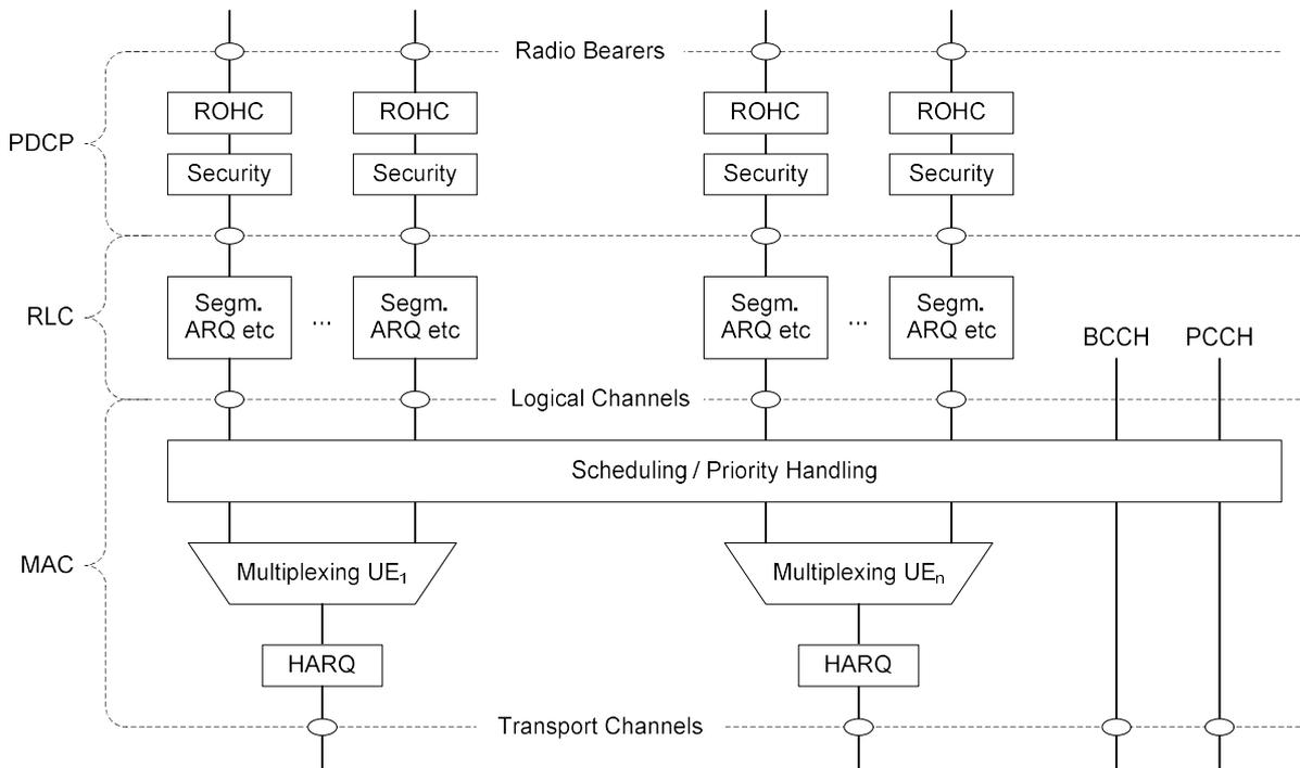
Figure 34: Downlink layer 2 structure [Ref. 7]
