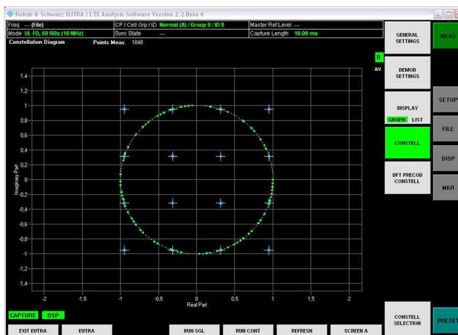
Figure 64: LTE uplink constellation diagram (16QAM)
