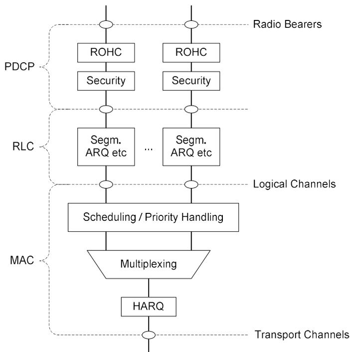
Figure 35: Uplink layer 2 structure [Ref. 7]
