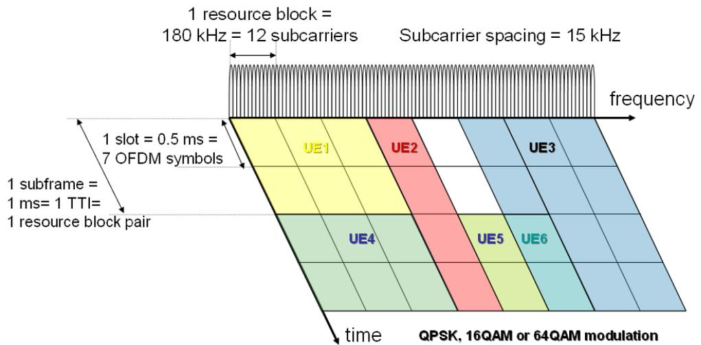
Figure 8: OFDMA time-frequency multiplexing (example for normal cyclic prefix)
