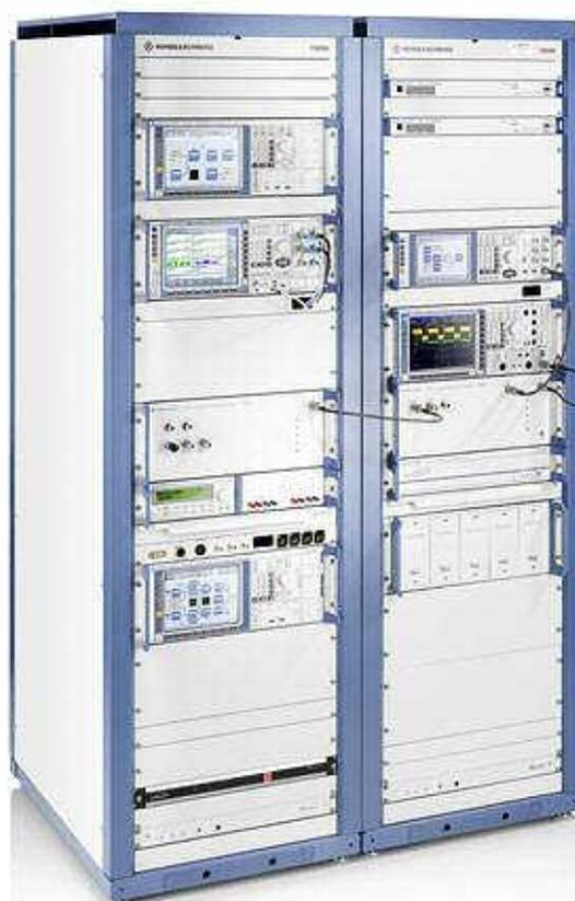
Figure 74: R&S®TS8980FTA with TV Interferers SFE100 (option for network operator specific testing)
