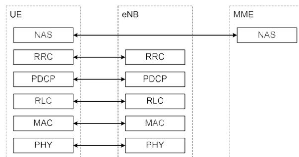
**Figure 31: Control plane protocol stack [Ref. 7]**
