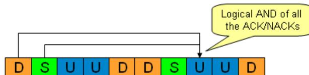
Figure 15: ACK/NACK bundling in TD-LTE
