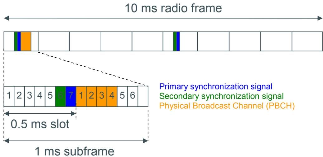
Figure 13: Primary/secondary synchronization signal and PBCH structure (frame structure type 1 / FDD, normal cyclic prefix)
