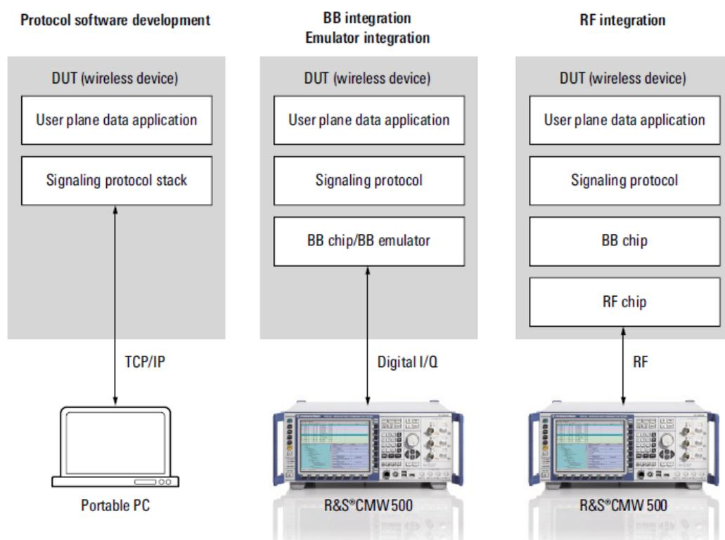
**Figure 69: R&S® CMW500 provides different interfaces to do protocol testing**
