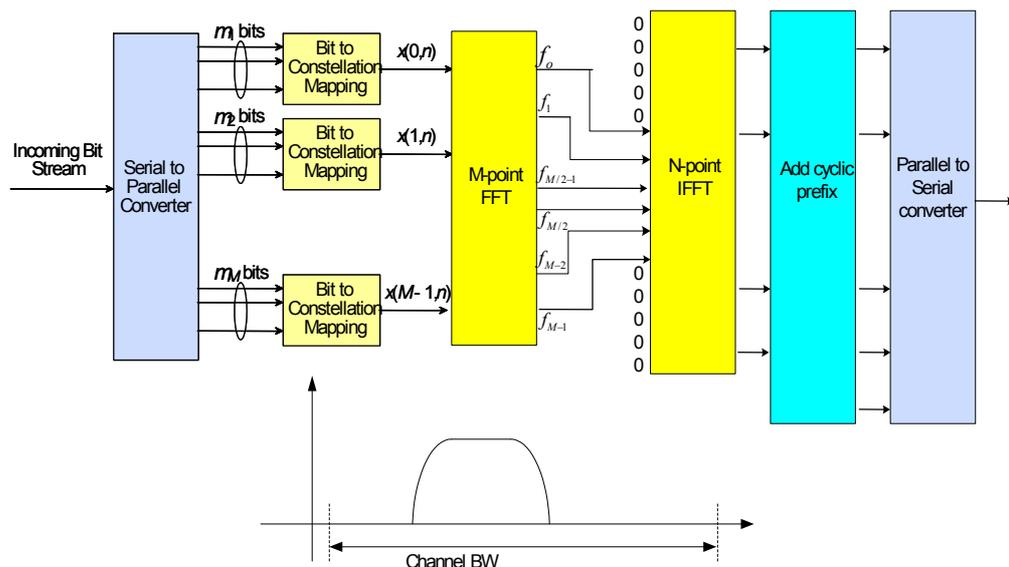
Figure 16: Block diagram of DFT-s-OFDM (localized transmission)
