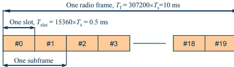
Figure 5: Frame structure type 1 [Ref. 3]
