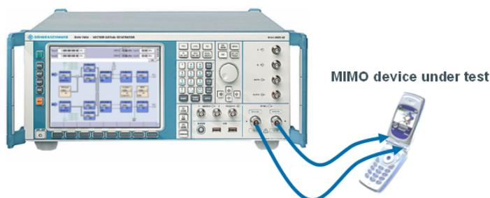
**Figure 66: Downlink MIMO receiver test: Signal generator SMU200A provides LTE downlink signals from two transmit antennas including channel simulation**
