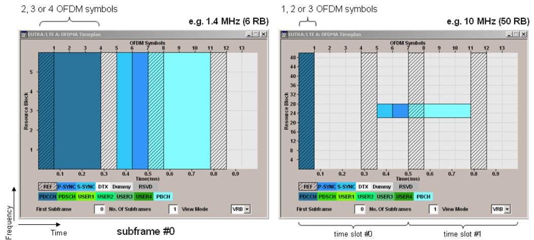
Figure 9: Number of OFDM symbols used for PDCCH are depending on bandwidth
