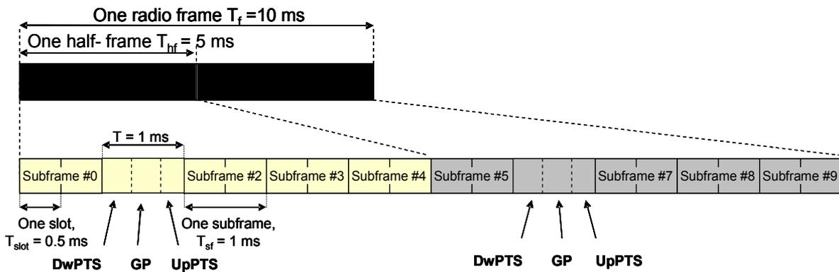
Figure 6: Frame structure type 2 (for 5 ms switch-point periodicity) [Ref. 3]
