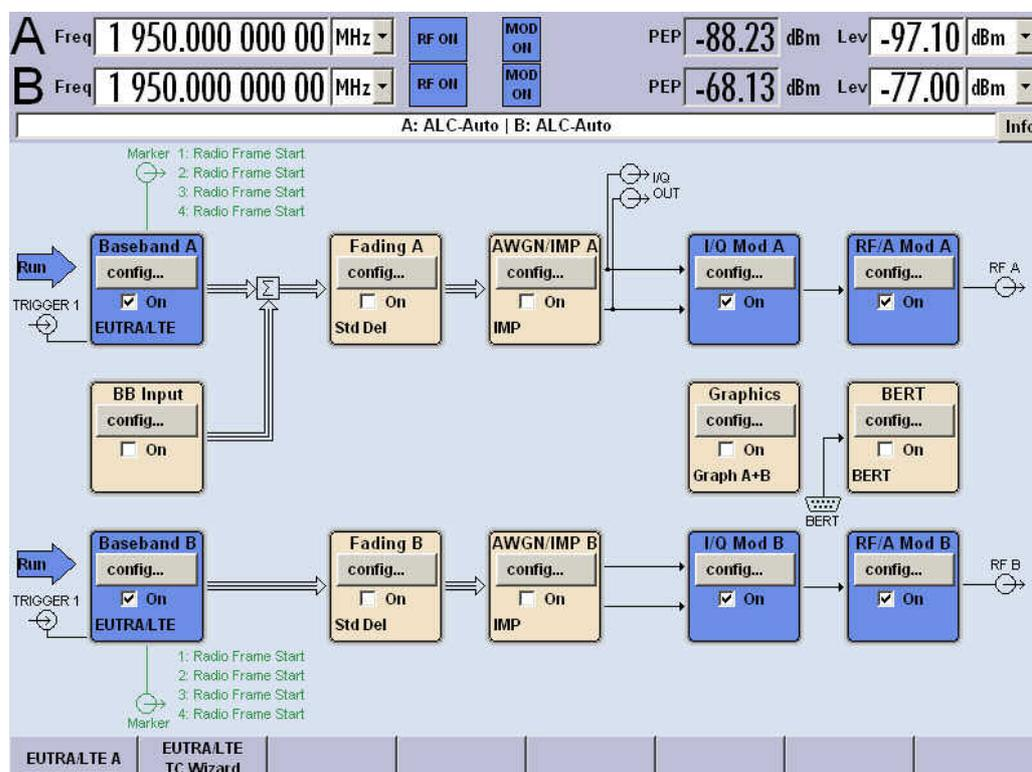
Figure 47: Block diagram SMU200A for In-Channel Selectivity according to TS 36.141 [Ref.16]
