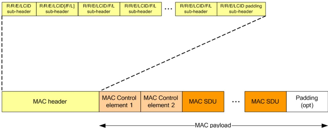
Figure 38: Structure of MAC PDU [Ref. 10]
