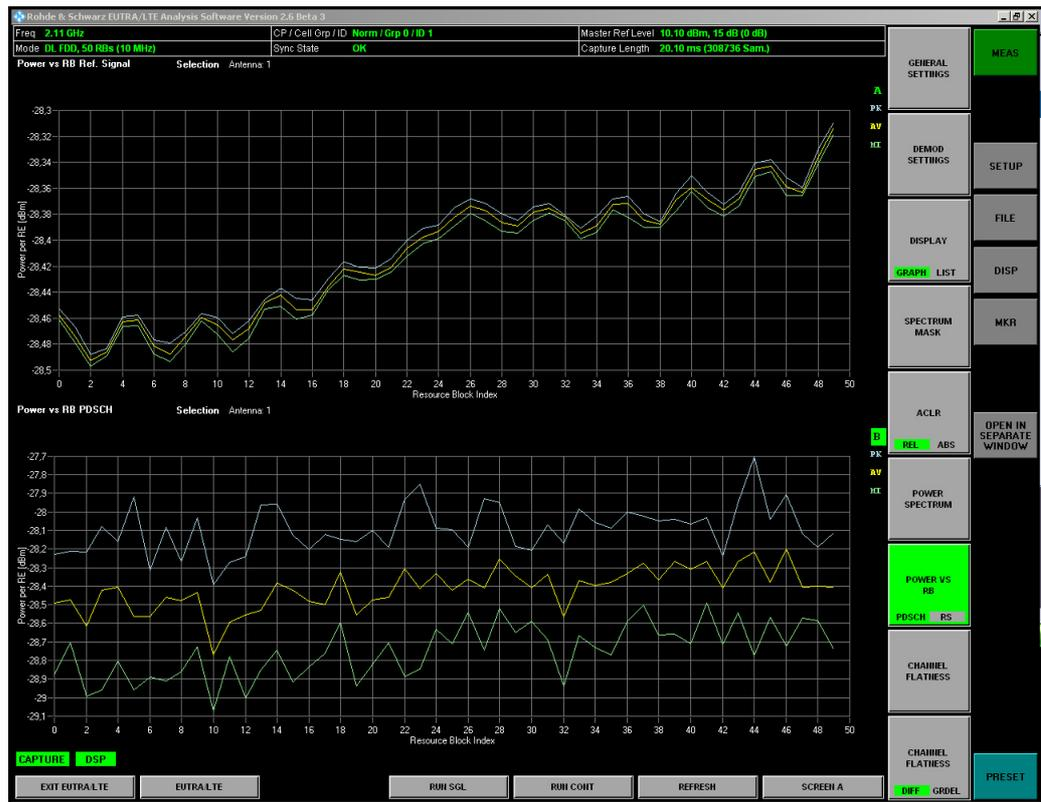
Figure 42: Power vs. RB Reference Signal and RB PDSCH (E-TM3.1, 10 MHz)
