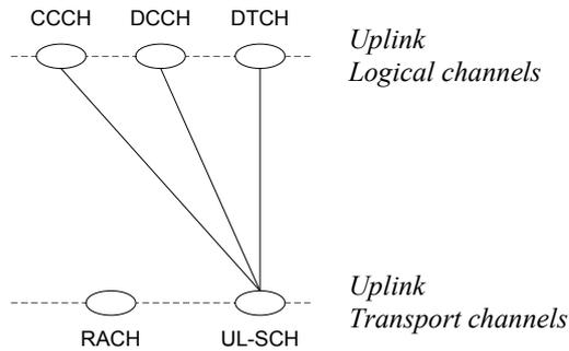
Figure 37: Mapping between UL logical and transport channels [Ref. 10]
