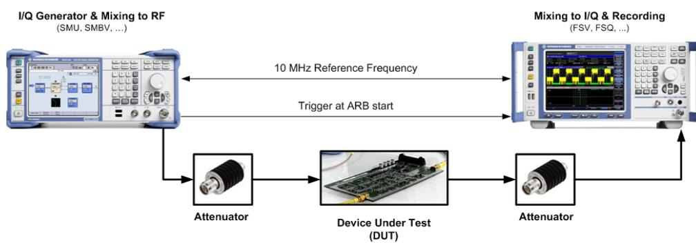
**Figure 40: R&S®FS-K130PC distortion analysis software – basic measurement setup**
