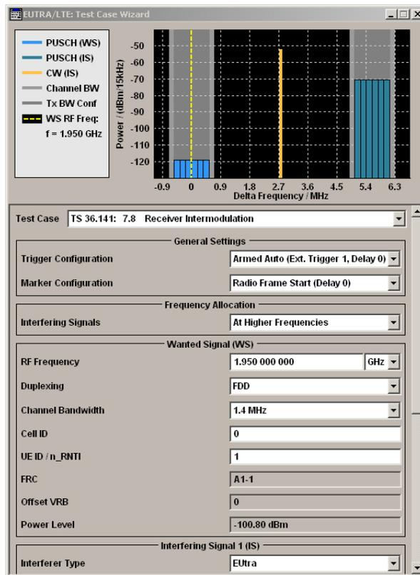
Figure 49: LTE test case wizard, configuring receiver intermodulation test acc. to TS 36.141 [Ref. 16]
