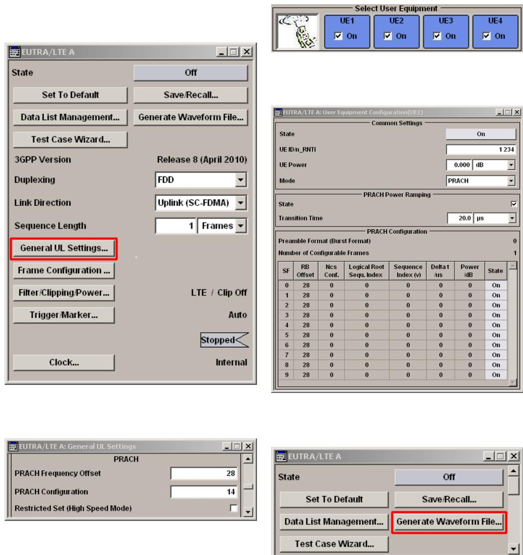
Figure 51: Basic parameter for PRACH overload testing with R&S®SMU200A Vector Signal Generator
