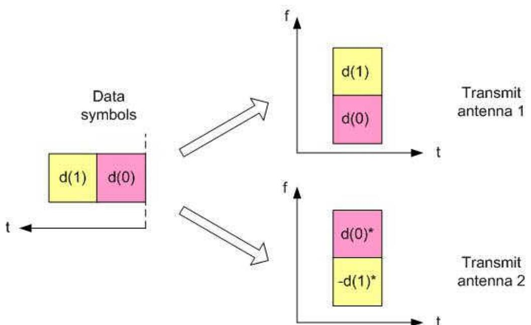
Figure 27: Transmit diversity (SFBC) principle
