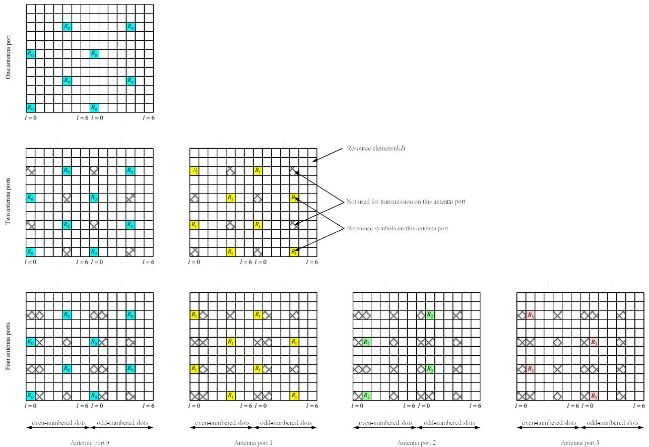
Figure 12: Downlink reference signal structure (normal cyclic prefix) [Ref. 3]
