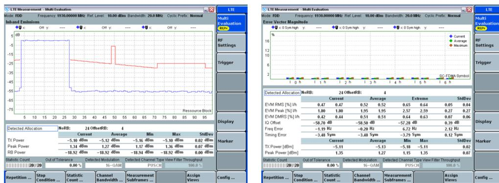
Figure 62: In-band emission (left) and EVM versus symbol measurement (right) [Ref. 18]
