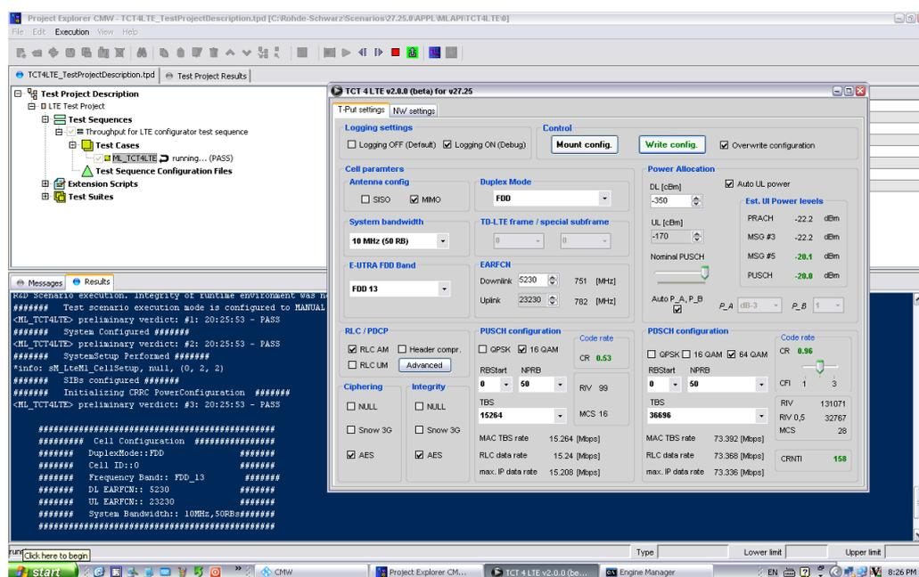
Figure 75: Throughput Configuration Tool for LTE (TCT4LTE) for R&S CMW500 LTE Protocol Tester
