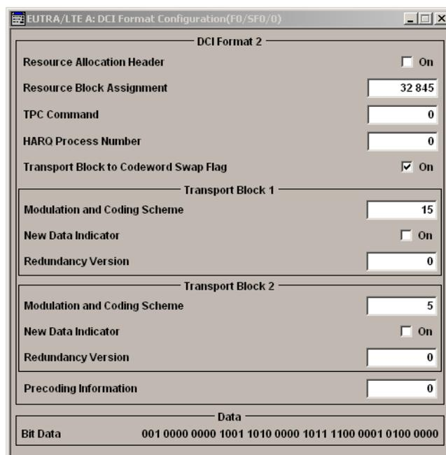
Figure 68: Configuration of DCI format 2 on R&S@SMU200A Vector Signal Generator
