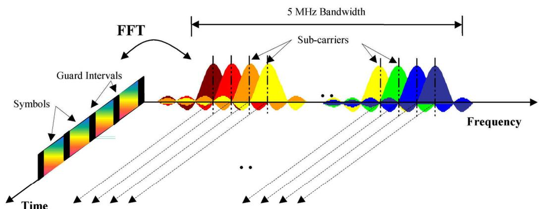
Figure 2: Frequency-time representation of an OFDM Signal [Ref. 2]
