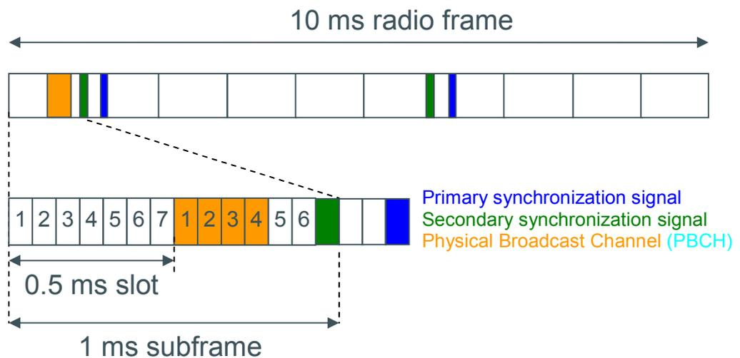
Figure 14: Primary/secondary synchronization signal and PBCH structure (frame structure type 2 / TDD, normal cyclic prefix)
