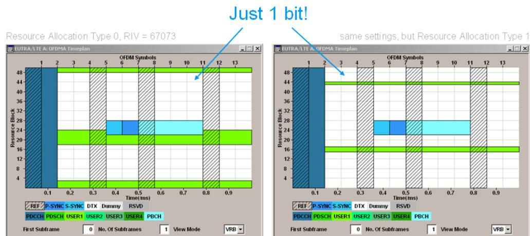
Figure 11: Difference between Resource Allocation Type 0 (left) and Type 1 (right)
