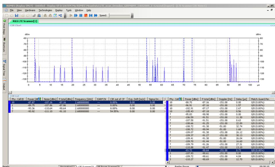
Figure 82: Channel Impulse Response (CIR) measurement displayed in R&S® ROMES
