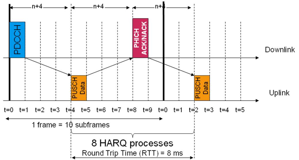
Figure 24: PHICH principle
