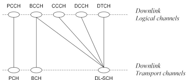
**Figure 36: Mapping between DL logical and transport channels [Ref. 10]**
