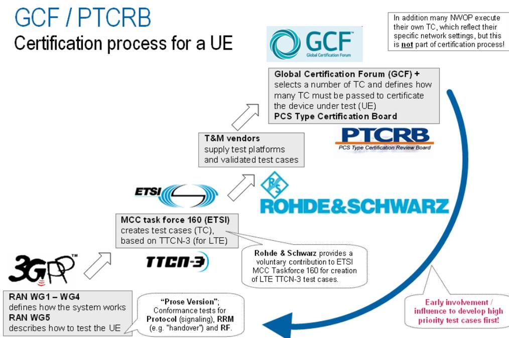
Figure 71: General work-flow of UE certification process, example LTE
