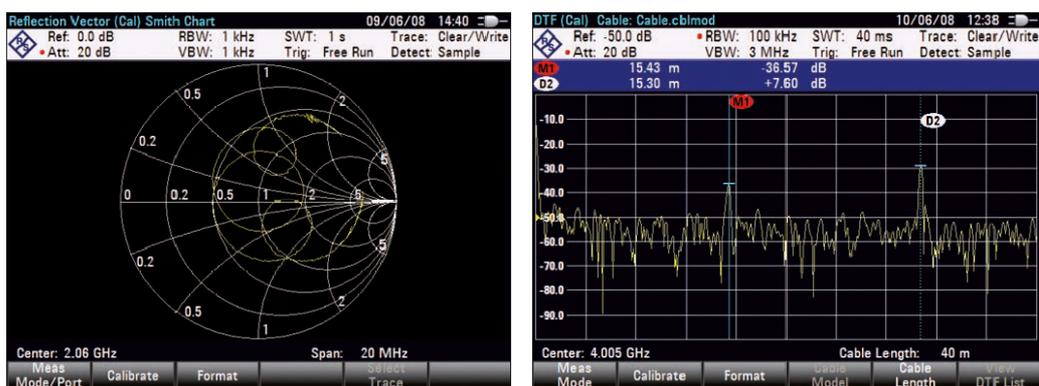
**Figure 85: Vector network analysis: measurement with Smith chart; Distance-to-fault measurements (DTF)**
