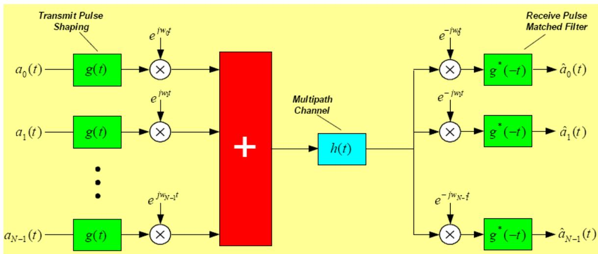
Figure 9.3.1. Basic Architecture of an OFDM System
