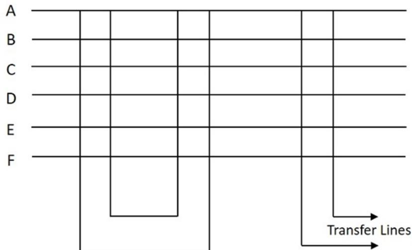
The switch shown in the above figure is blocking both internally and externally with two simultaneous internal and two simultaneous external calls. The number of Crosspoint switches in this case is  $N(2K+L)$ , where  $N$  is the number of subscribers,  $L$  is the number of transfer lines and  $K$  is the number of simultaneous calls that can be supported locally.
