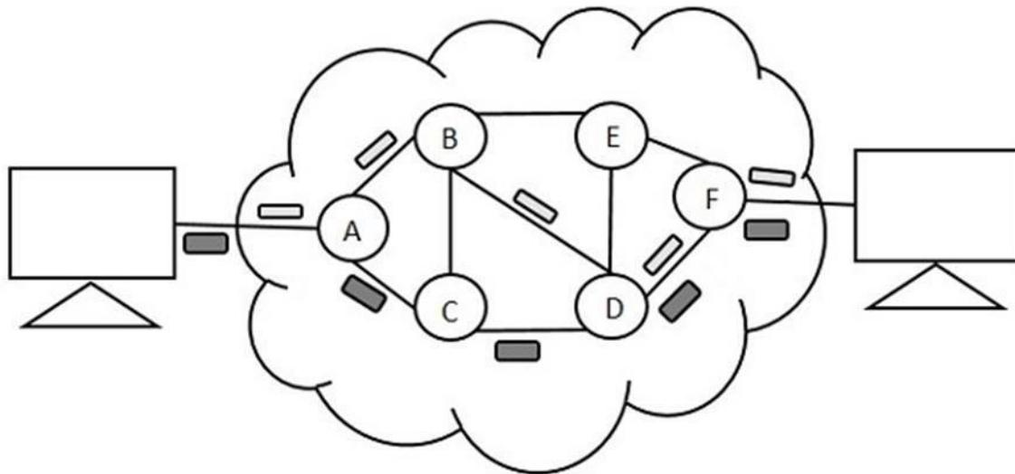
In this technique, the data is stored and forwarded. The technique is also called the **Store-and-Forward** technique. This technique was considered a substitute to circuit switching. But the transmission delay that followed the end to end delay of message transmission added to the propagation delay and slowed down the entire process.
