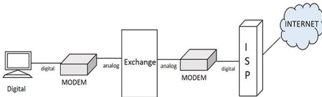
The above figure shows that the digital signals have to be converted into analog and analog signals to digital using modem during the whole path. What if the digital information at one end reaches to the other end in the same mode, without all these connections? It is this basic idea that led to the development of **ISDN**.
