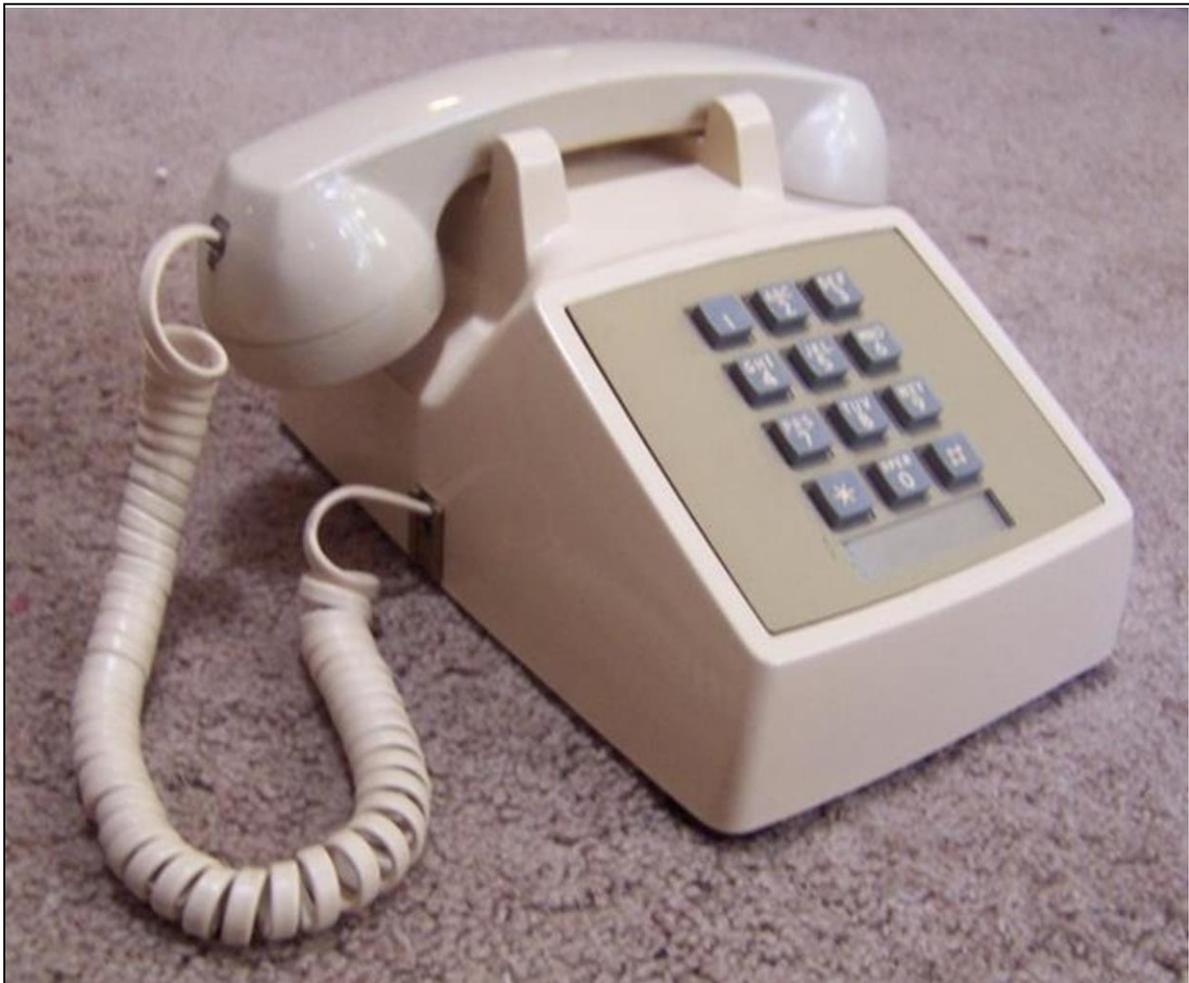
The above figure will help you understand that the rotary dial is replaced with a push button keyboard, where the buttons, if touched to –press|| the button will generate frequencies
