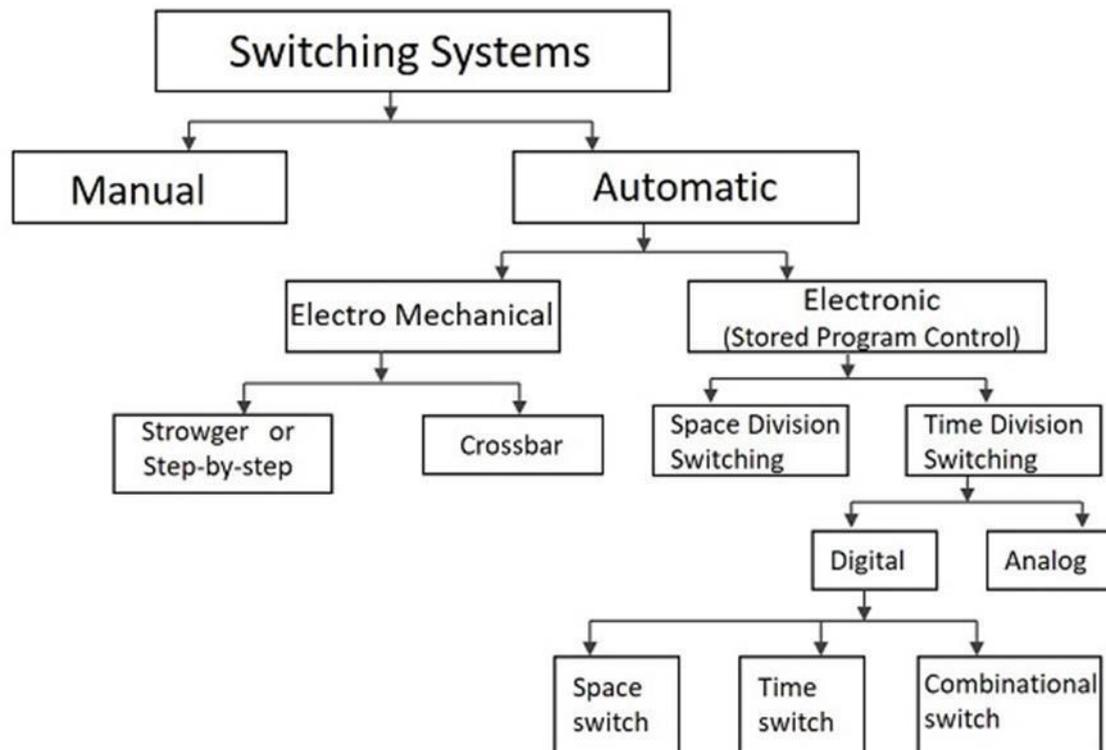
The switching systems in the early stages were operated **manually**. The connections were made by the operators at the telephone exchanges in order to establish a connection. To minimize the disadvantages of manual operation, automatic switching systems were introduced.
