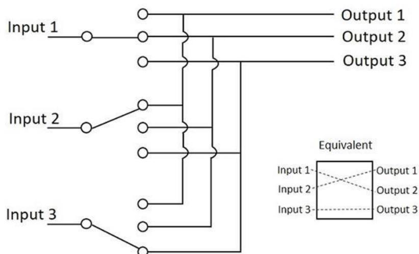
Though the space division switching was developed for the analog environment, it has been carried over to digital communication as well. This requires separate physical path for each signal connection, and uses metallic or semiconductor gates.
