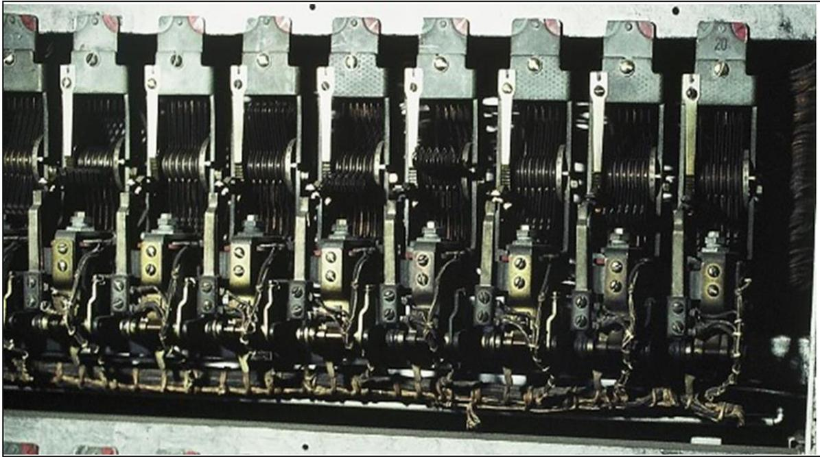
Thus, the wiper assembly establishes the call; after completion of which it comes back to the home position. For this purpose, the rotary magnet is operated by the current and thus the wiper assembly moves through the remaining contacts of the level. A restoring spring forces the wiper assembly to drop vertically and then return horizontally to the home position.
