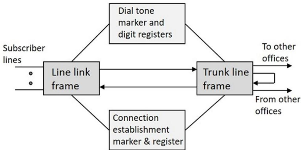
The call processing in a Crossbar exchange is done in three stages, named as Pre- Selection, Group Selection and Line Selection.
