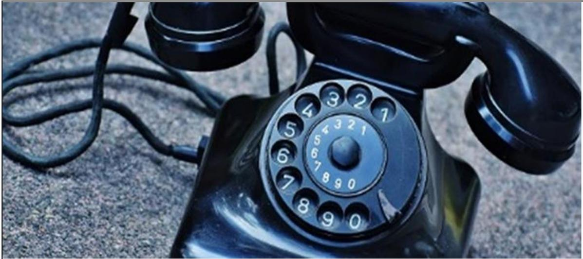
The dial is operated by placing the finger in the hole appropriate to the digit to be dialed. Now, drawing the fingerplate round in the clockwise direction to the finger stop position and letting the dial free by withdrawing the finger, makes a number dialed. The fingerplate and the associated mechanism now return to the rest position under the influence of a spring. The dial is ready for the next number.
