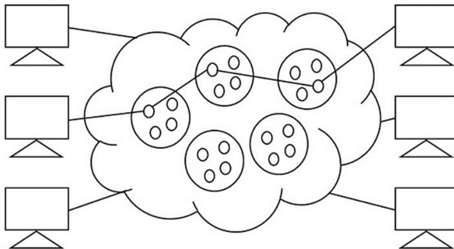
Circuit switching was designed for voice applications. Telephone is the best suitable example of circuit switching. Before a user can make a call, a virtual path between the called subscriber and the calling subscriber is established over the network.
