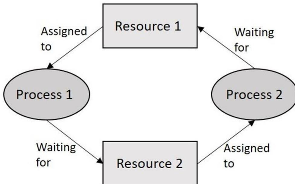
If two or more processes in a semaphore wait indefinitely for a resource and does not get zero to return to the block state, while other processes wait in the blocked state for the use of the same resource while none could use the resource but wait, such a state is called the **Deadlock State**.
