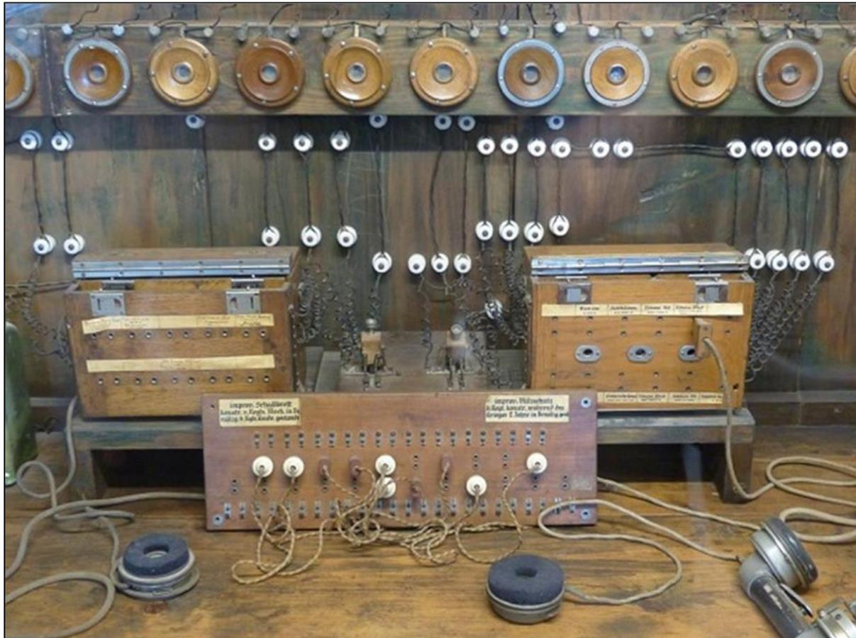
The above figure shows an early model of the PBX system. The PBX is usually operated and owned by the local office where the users are connected through it within that limited area.
