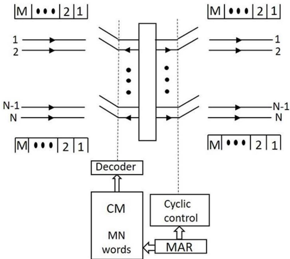
The interchange of time slots is not possible in time division switching, as the incoming time slot transfers the data to its dedicated output time slot only. Hence, time multiplexed switches do not provide full availability.
