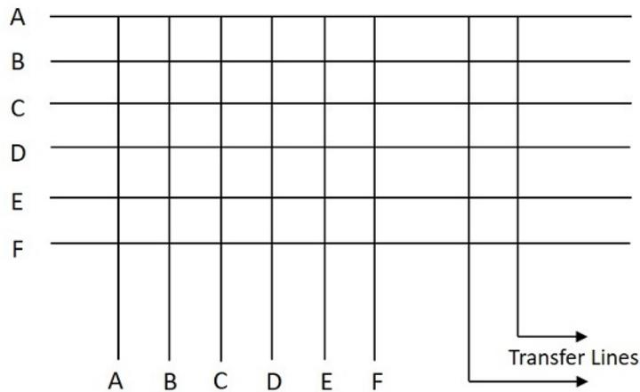
The switch shown in internal non-blocking has two transfer lines. The number of Crosspoint switches in this case is  $N(N+L)$ , where  $N$  is the number of subscribers,  $L$  is the number of transfer lines.
