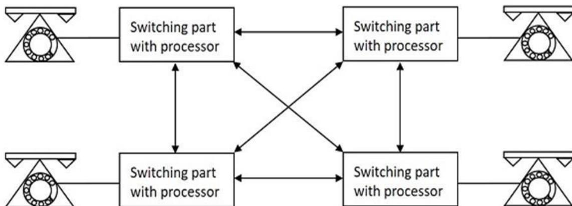
The exchange environment in vertical decomposition is divided into several blocks and each block is assigned to a processor that performs all the control functions that are related to specific block of equipment, whereas each processor in horizontal decomposition performs one or some of the exchange control functions.
