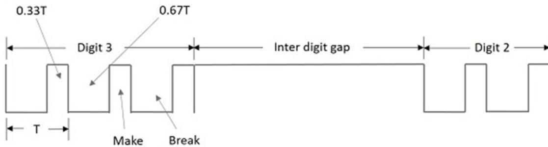
The above figure shows the pulsating pattern. The pulse rate is usually 10 pulses per second with a 10 percent of tolerance. The gap between the digits, which is called the Inter-digit gap is at least 200ms.
