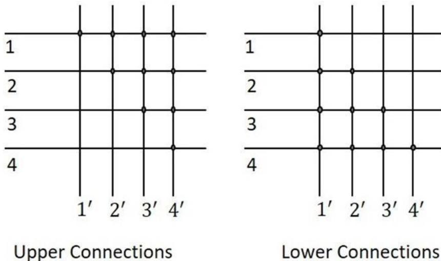
Now, the diagonal portions are the Crosspoints connecting to the same subscriber again. A line that is already connected to the terminal has no need of connecting it again to the same terminal. Hence, the diagonal points are also not necessary.
