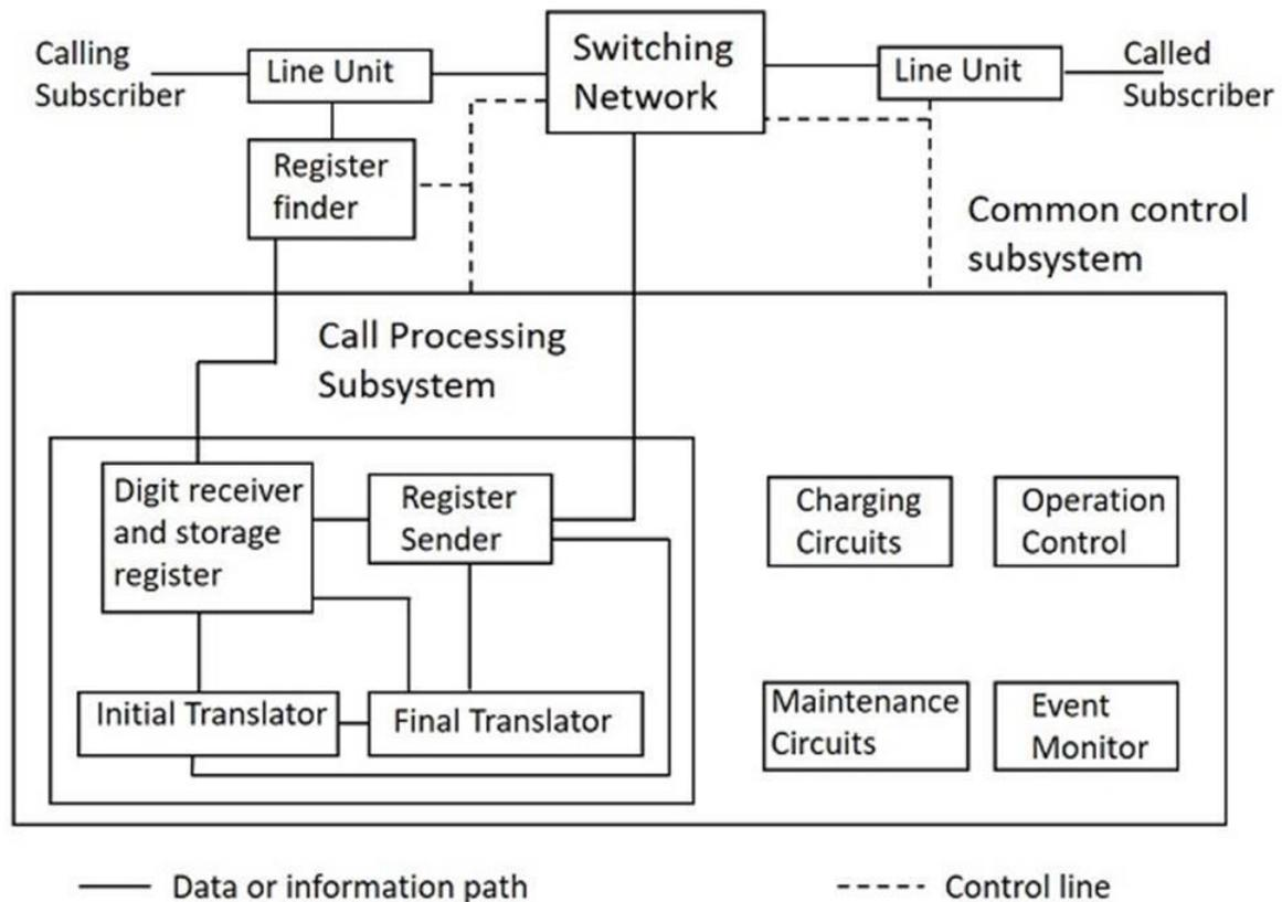
The above block diagram is a simple indication of the common control switching system. The control functions in a switching system can be categorized as the following.
