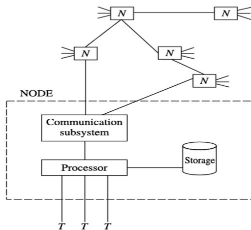
The network moves the user information from node to node. One such movement is called a hop. Since the communication links are used one at a time between any two nodes, line speeds can be utilised efficiently. S&F switching may be classified as:
