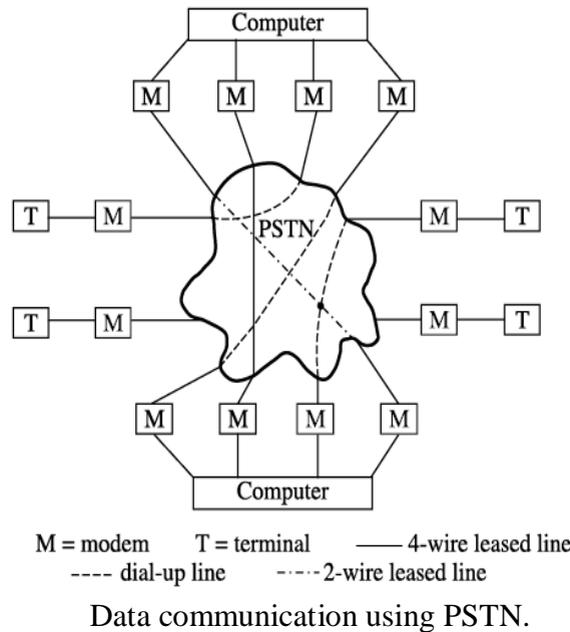
In a PSTN, a connection may be established using a dial-up facility or a dedicated non-switched leased line. A 2-wire or 4-wire leased line may be used. The modems usually have automatic dialling and answer facility which is useful when working with dial-up line. Modems are driven by a communication software package that runs on the terminal or the personal computer of the user. The transmission may be half-duplex or
