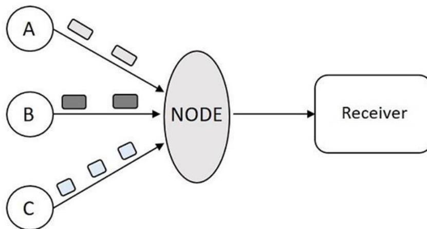
In the above figure, when the data packets arrive at Node from the senders A, B and C then the node cannot transmit the data to the receiver at a faster rate. There occurs a delay in transmission or may be data loss due to heavy congestion.
