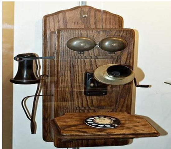
When you see the telephone in the above figure, the dialer part and the microphone are connected to a stationary wooden plank; and the speaker to listen, was connected by a wire at the side. The top portion of the telephone has two bells connected - these bells ring when there is an incoming call. This is one of the earlier models of the telephone.
