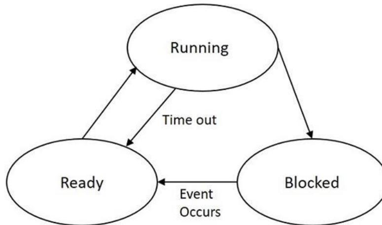
While some processes are in the running state, some will be in the ready state while others are blocked up. The processes in the ready list will be according to the priorities. The blocked processes are unordered and they unblock in the order in which the events are waiting to occur. If a process is not executed and waits for some other instruction or resource, the processor time is saved by pushing such process to the ready list and will be unblocked when its priority is high.
