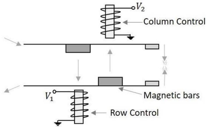
Once energized, the electromagnets pull the small magnetic slabs present on the bars. The column control electromagnet pulls the magnet on the lower bar, while the row control
