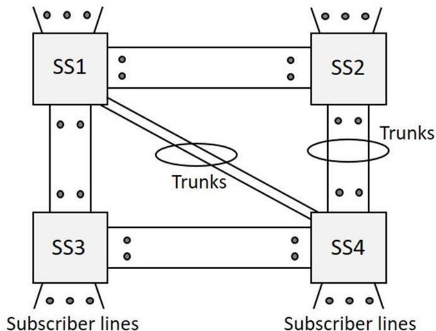
From the early to the later stages of the 20<sup>th</sup> Century (1900-80), when a person needed to make a distant call, the call was first routed to the operator at the nearest switching center and then the number and location of the called subscriber was noted down. Here, the job of the operator was to establish a call to the remote switching center and then recall the calling subscriber to establish the connection. This system of making calls was called the **Trunk call** system.
