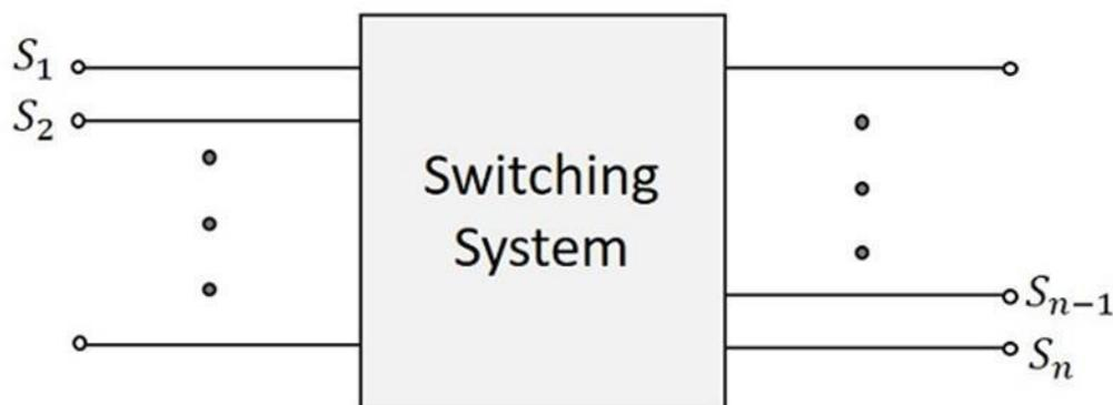
With the introduction of switching systems, the need for traditional connections between the subscribers reduced. All the subscribers need to **have a connection with the switching system**, which makes or breaks any connection, requested by the calling subscriber. The switching system, which is also called the **Telephone Exchange**, takes care of establishing the calls. Hence, the total number of such links is equal to the number of subscribers connected to the system.
