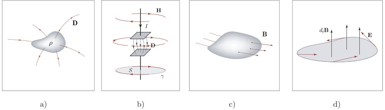
Figure 1.5: Schematic on the integral form of Maxwell's equations. a) Gauß's law, b) circulation of the magnetic field, c) absence of magnetic charges, d) law of induction
