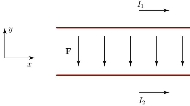
Figure 2.2: Two infinite wires exerting a force on each other
