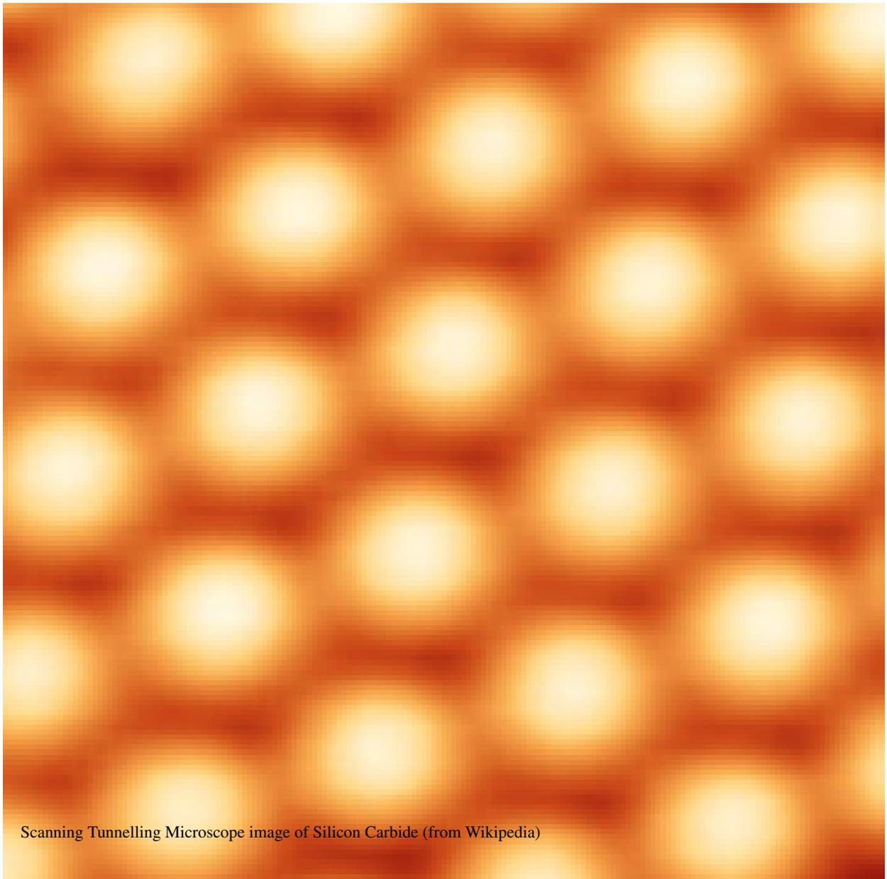
Scanning Tunnelling Microscope image of Silicon Carbide (from Wikipedia)
