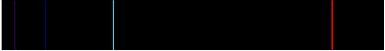
Atoms, excited by an ionizing potential, emit not a continuous rainbow of colors but a discrete set of colors - the atomic emission spectrum. Each atom has a characteristic spectrum. We are ready to confront this last mystery of the 1800s.
