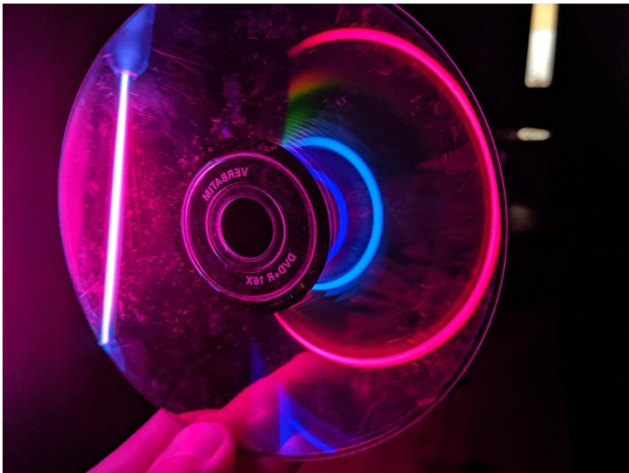
The emission spectrum of Hydrogen gas, revealed by scattering off an optical disk (above) and shown more clearly all in a plane (below). Emission spectra were first observed by Angstrom.
