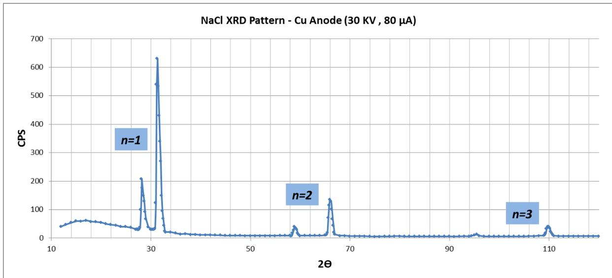
The copper x-ray emitter generates two x-ray wavelengths:  $\text{Cu } K\alpha$ , with  $\lambda = 0.15406\text{nm}$ , and  $K\beta$ , with  $\lambda = 0.13923\text{nm}$ . Using the above data, we can estimate  $d = 0.28\text{nm}$ . . . the spacing in NaCl is about the same scale as the x-ray wavelengths.
