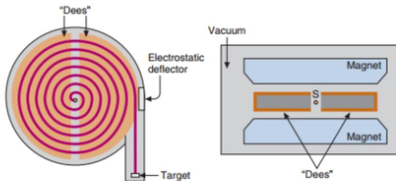
**FIGURE 5-3** Schematic representation of a positive ion cyclotron: top (*left*) and side (*right*) views. The accelerating voltage is applied by a high-frequency oscillator to the two "dees." S is a source of positive ions.
