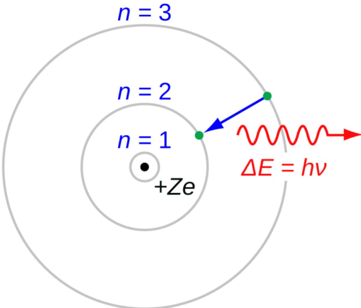
The atom conserves energy. For an electron to go to a wider orbit, it must absorb energy; a photon of the right frequency and wavelength can do that. To drop to a lower orbit, it must release energy; emitting a photon of a specific wavelength and frequency will do that, too.
