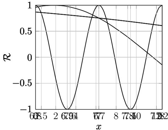
Measuring the *position* of a free particle boils down to determining where it is along the x-axis. Measuring the *momentum* of the same particle boils down to determining the curvature of the wave at a given point, e.g.  $\partial^2/\partial x^2$  (which, when applied to the wave function, returns  $k^2$ , the square of the wave number, which provides a measure of the momentum).
