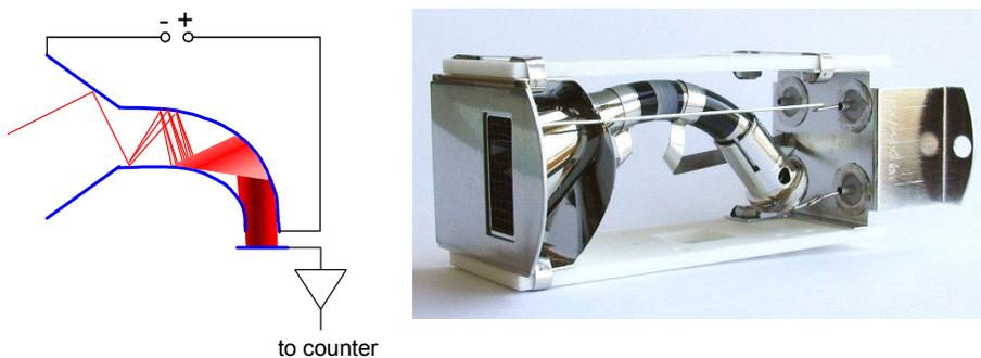
Figure 43. Channeltron® detector.
