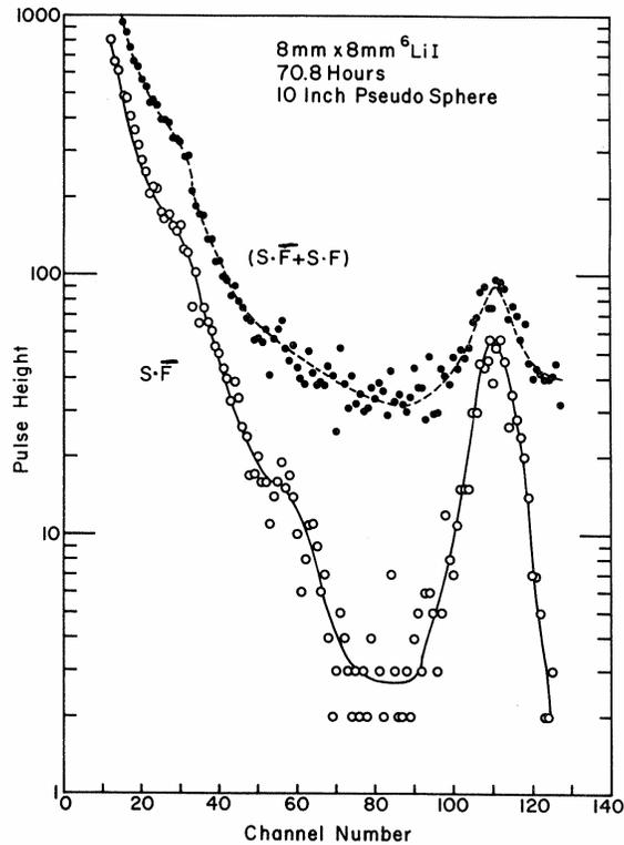
Fig. 9.7 Pulse height spectra obtained using the phoswich shown in Fig. 9.6 in a natural background radiation field. The **upper curve** (filled circles) is a spectrum of all slow pulses (slow with fast and slow without fast). The **lower curve** (open circles) is a spectrum of slow pulses not accompanied by fast pulses, interpreted to be due to neutrons. [Reproduced from (Aw73).]
