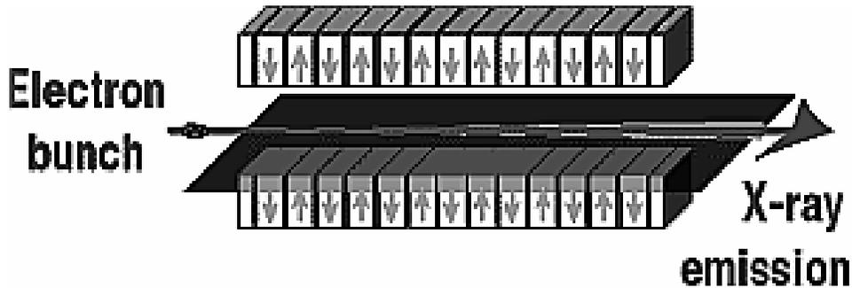
Fig. B.4 Sketch of a typical insertion device. [Provided by courtesy of J. Liu and V. Vylet.]
