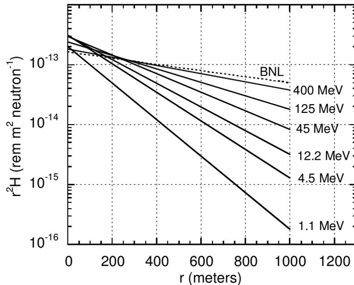
Fig. 5.14 Variation of dose equivalent with distance  $r$  for  $1/E$  neutron spectra with different upper energies. The ordinate is dose equivalent  $H$  times  $r^2$ . The curve labeled "BNL" is the result of a measurement at the Brookhaven National Laboratory Alternating Gradient Synchrotron, a 30 GeV proton accelerator. [Adapted from (St84a).]
