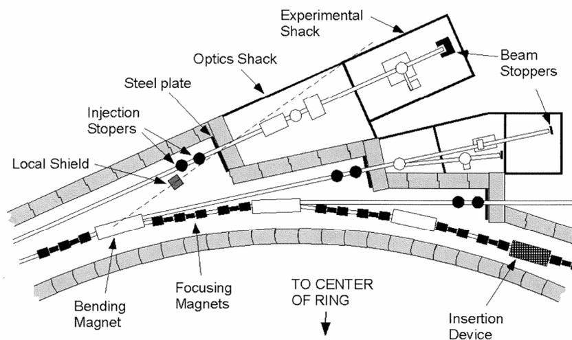
Fig. B.7 Typical synchrotron radiation facility experimental installation. The storage ring is at the bottom of the frame. So called “ratchet-walls” separate the experimental installations from the main storage ring. [Adapted from (NC03).]
