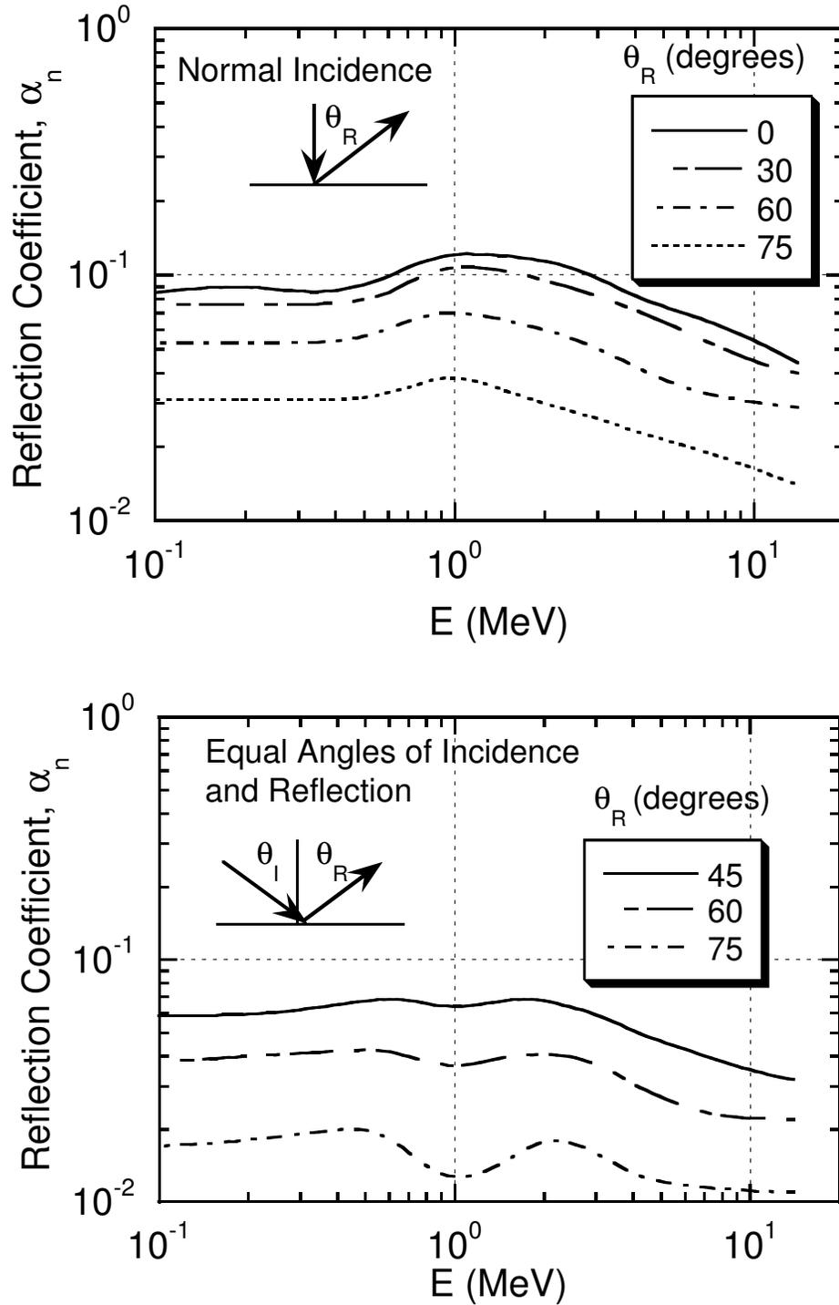
Fig. 5.2 Reflection coefficients,  $\alpha_n$ , for monoenergetic NEUTRONS incident on ordinary concrete as a function of incident neutron energy for several angles of reflection assuming normal incidence (**top frame**) and for equal angles of incidence and reflection ( $\theta_i = \theta_R$ ) (**bottom frame**). [Adapted from (NC03) and references cited therein.]
