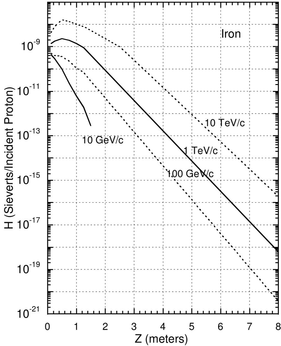
Fig. 4.25 Dose equivalent per proton,  $H$ , on the longitudinal axis,  $Z$ , as a function of depth  $Z$  in the shield for proton-induced cascades in IRON of density  $7.2 \text{ g cm}^{-3}$ . The curves are the result of CASIM calculations for incident proton momenta of 100 GeV/c, 1 TeV/c, and 10 TeV/c and FLUKA results for 10 GeV/c. [Adapted from (Sc90).]
