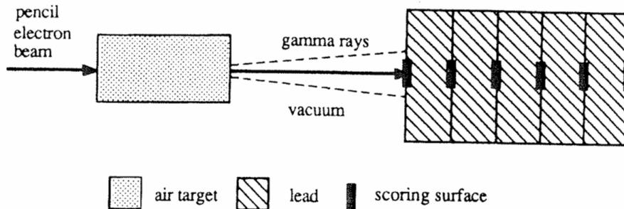
Fig. B.8 Geometry considered by Tromba and Rindi in their Monte Carlo calculations of gas bremsstrahlung. An electron pencil beam crosses an air target. The bremsstrahlung photons are attenuated in lead. The number of photons and the relative dose are scored on a small surface (about  $1 \text{ cm}^2$ ), smaller than the photon-beam angular opening at different depths in the lead. [Adapted from (Tr90).]
