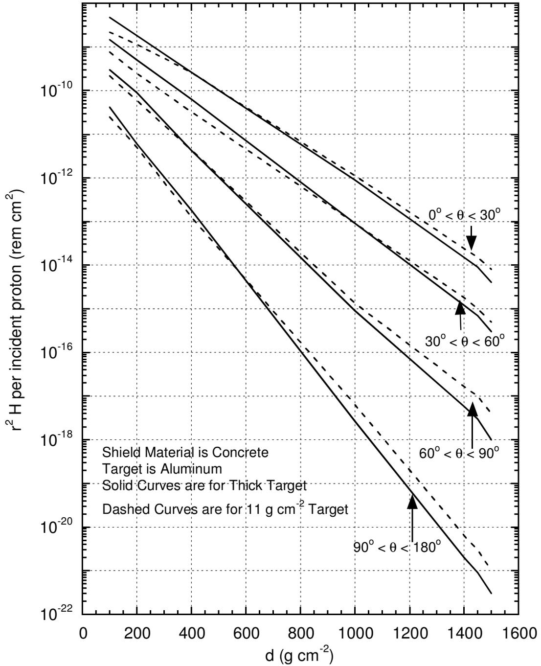
Fig. 4.23 HETC calculations of  $r^2H$  as a function of CONCRETE shield thickness,  $d$ , averaged over several intervals of  $\theta$  for 200 MeV protons incident on an aluminum target centered in a spherical shield. [Adapted from (AI75).]
