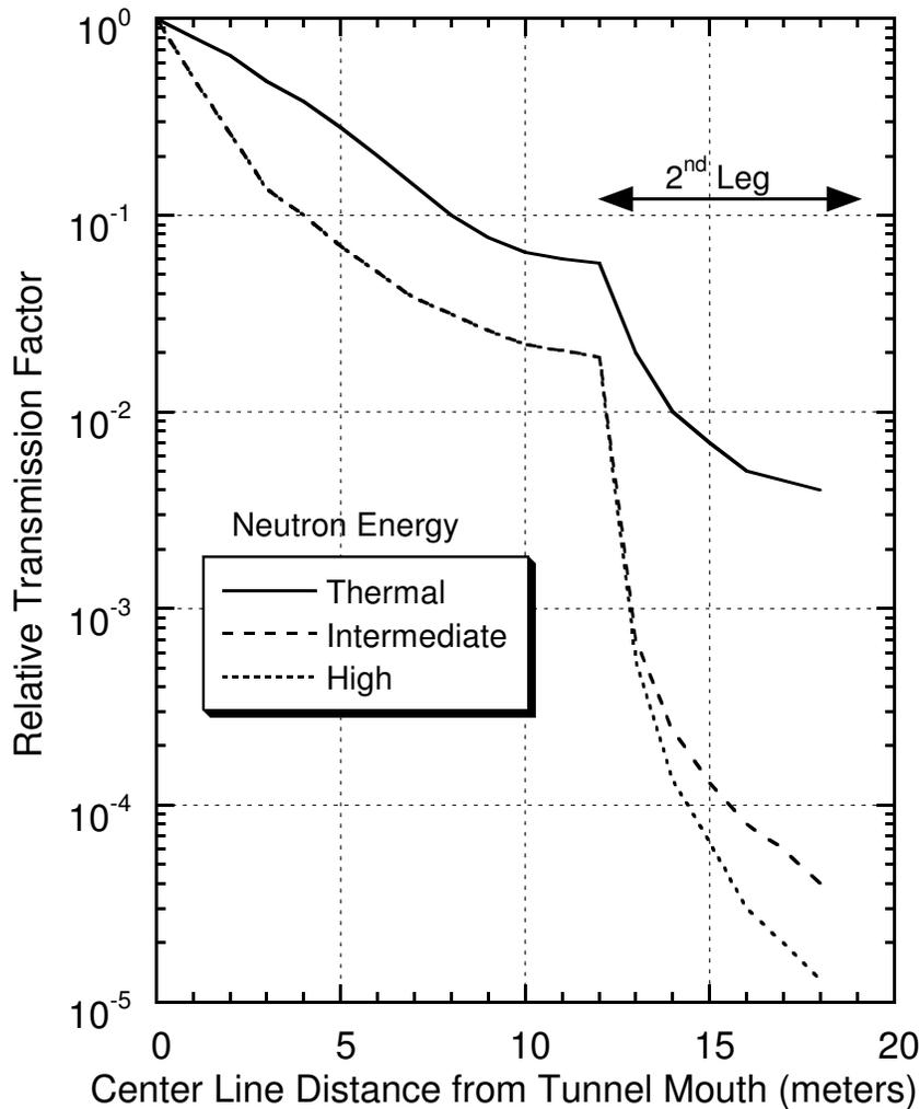
Fig. 5.7 Relative transmission of particle flux density along a two-legged labyrinth using threshold detectors. The curve labeled "**thermal**" corresponds to the measured attenuation of thermal neutrons, the curve labeled "**intermediate**" corresponds to neutrons having energies between approximately 6 and 25 MeV while the curve labeled "**high**" corresponds to neutron energies above 20 MeV. [Adapted from (St73).]
