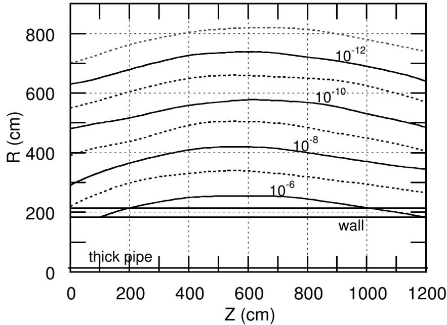
Fig. C3.c Contour plots of equal star density (stars cm<sup>-3</sup>) per incident proton calculated using CASIM for a 1 TeV proton beam incident “head on” on a thick cylindrical iron pipe of 30.48 cm outside diameter with 1.27 cm thick walls. The results were averaged over azimuth and the pipe was centered in a cylindrical tunnel 182 cm in radius. The concrete wall was 30.48 cm thick and was surrounded by soil. [Adapted from (Co82b).]
