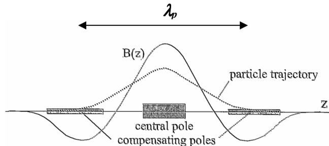
Fig. B.3 Schematic of a wavelength shifter showing the three magnets involved; the magnetic field strength,  $B(z)$ , as a function of longitudinal coordinate  $z$ ; and the electron trajectory.  $\lambda_p$  is the length of a **period** of group of such magnets, here consisting of a pair. Since the pole pieces are typically short, the magnetic field strength may have an approximate sinusoidal dependence on  $z$  as depicted here. [Adapted from (Wi03).]
