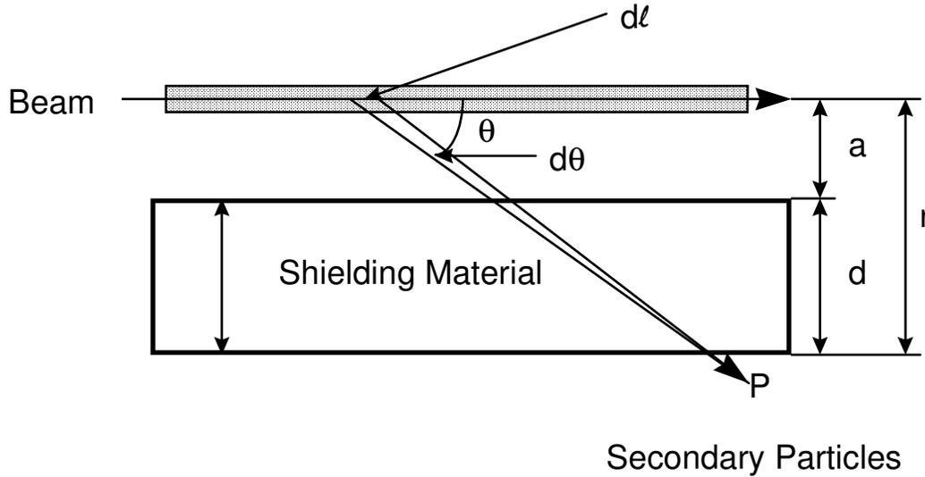
Figure 4.22 Variables of integration of Moyer point source result needed to obtain Moyer line source results. As in Fig. 4.21, the shielding of thickness  $d$  could be comprised of multiple layers of thickness  $\zeta$  mean free paths.
