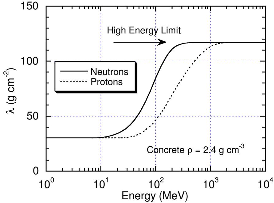
Fig. 4.17 The variation of the attenuation length  $\lambda$  for monoenergetic neutrons and protons in concrete shielding as a function of neutron energy. The high energy limit is  $117 \text{ g cm}^{-2}$ . [Adapted from (Th88).]
