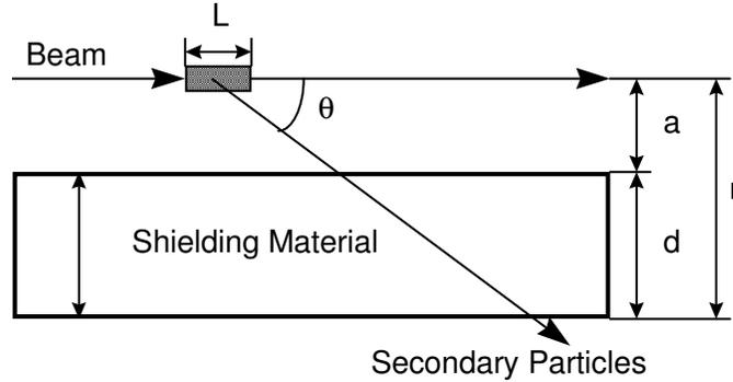
Fig. 3.11 Target and shielding geometry for the estimation of dose equivalent due to electron beam interactions with a target surrounded by a cylindrical shielding.  $L$  is the length of the target and the other parameters specify the geometry.
