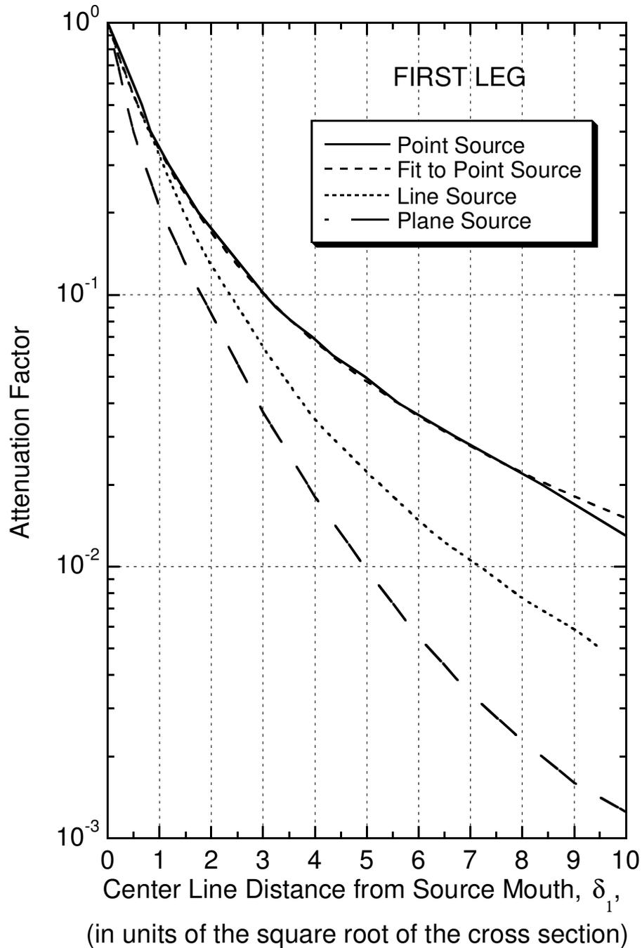
Fig. 5.6 Universal transmission curves for the first leg of a labyrinth as a function of normalized distance,  $\delta_1$  from the mouth. The fit for the point source curve represented by Eq. (5.4) is also included. The curve for a plane source is also suitable to use with an off-axis point source. [Adapted from (Go75) and (Co95).]
