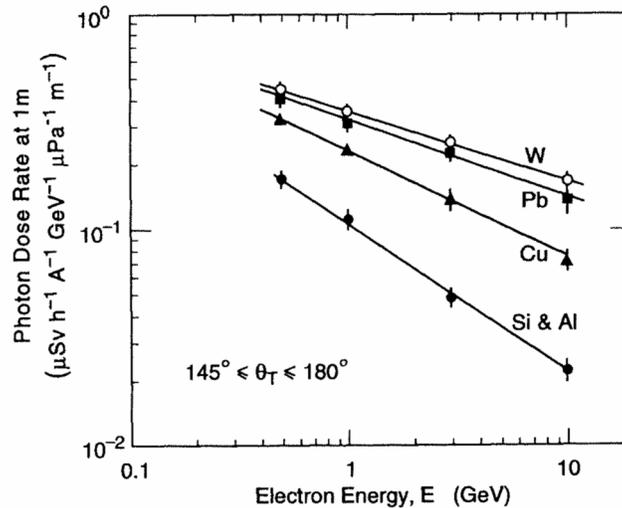
Fig. B.9 Secondary photon dose rate at 1 m lateral to large targets of various materials as a function of electron beam energy. The values are normalized to a beam current of 1 Ampere, per GeV beam energy, and an air path of 1 meter with a pressure of 1  $\mu\text{Pa}$  ( $= 7.50 \times 10^{-9}$  torr). [Adapted from (Li95).]
