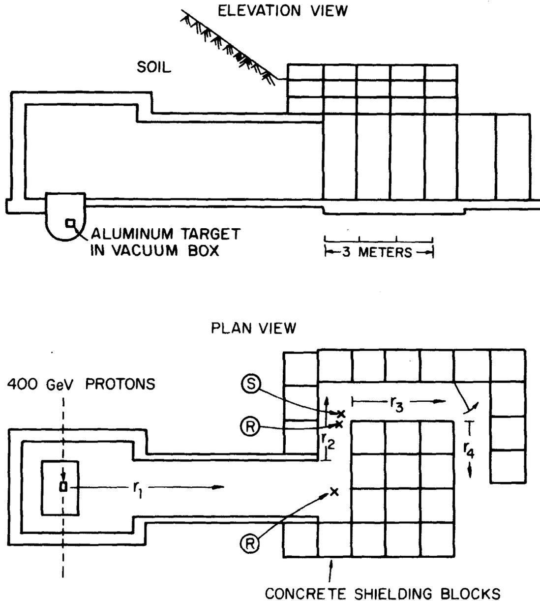
Fig. 5.9 Labyrinth enclosure in which 400 GeV protons interacted with an aluminum target located beneath the floor as shown. The neutron energy spectrum was measured at the location denoted "S" and the quality factor of the radiation field was measured at the locations denoted "R". [Adapted from (Co88).]
