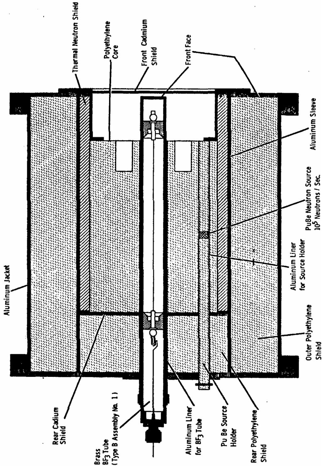
Fig. 9.10 Schematic diagram of a DePangher Long Counter. This version contains a built-in PuBe source, which is optional. The source would not be desirable in an instrument to be used in radiation fields near natural background. The dimensions and mass of this instrument are given in the text. [Reproduced from (DeP66).]
