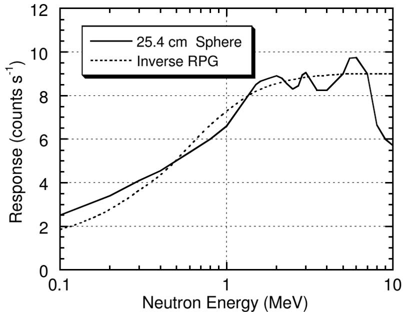
Fig. 9.8 Sensitivity of detector comprised of a 25.4 cm (10 in.) diameter moderating sphere surrounding a  $4 \times 4 \text{ mm}^2$  cylindrical LiI scintillator in  $\text{counts s}^{-1}$  at 40 cm distance from a source of  $10^6 \text{ neutrons s}^{-1}$ . Also shown is the relative dose equivalent per neutron labeled as "Inverse RPG". At thermal energies, the response was measured to be 0.227 compared with a value of 0.225 for the "Inverse RPG" curve (see text). [Adapted from (Ha62).]
