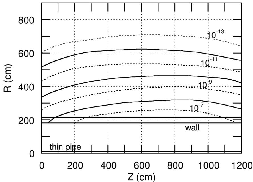
Fig. C3.b Contour plots of equal star density (stars  $\text{cm}^{-3}$ ) per incident proton calculated using CASIM for a 1 TeV proton beam incident “head on” on a thin cylindrical aluminum pipe of 10.16 cm outside diameter with 0.318 cm thick walls. The results were averaged over azimuth and the pipe was centered in a cylindrical tunnel 182 cm in radius. The concrete wall was 30.48 cm thick and was surrounded by soil. [Adapted from (Co82b).]
