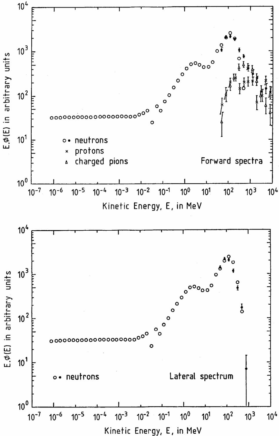
Fig. 6.4 Neutron energy spectra outside of a concrete shield at a high energy proton accelerator at forward angles (**upper frame**) and at large angles (**lower frame**). The open circles represent the calculations of O'Brien (OB71) while the other symbols represent the calculations of Höfert and Stevenson. [Adapted from (Hö84a).]
