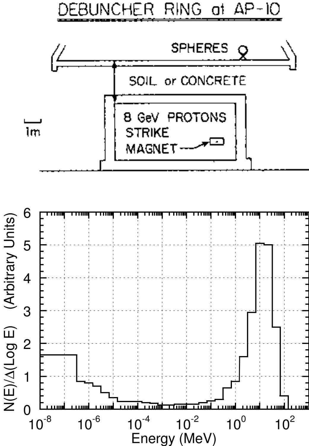
Fig. 6.5 Neutron energy spectrum (**lower frame**) obtained external to a beam enclosure (**upper frame**) in which 8 GeV protons struck the yoke of a magnet. The site was the Fermilab Debuncher Ring. The normalization of the spectrum is arbitrary. [Adapted from (Co88).]
