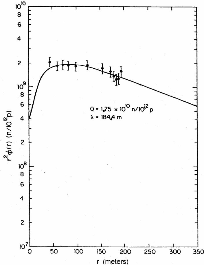
Fig. 5.17 The product of  $r^2$  and the neutron fluence  $\phi(r)$  per  $10^{12}$  protons incident on a target as a function of the distance from the source  $r$ . The source is that described in connection with Fig. 6.8. The smooth curve is a fit to Eq. (5.17) with parameters  $\lambda = 184.4$  m and  $Q = 1.74 \times 10^{10}$  neutrons per  $10^{12}$  protons. [Reproduced from (El86).]
