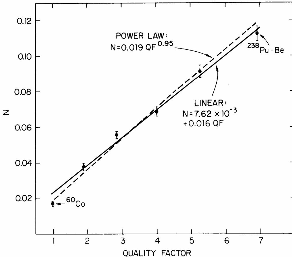
Fig. 9.15 Response of a recombination chamber as a function of quality factor  $Q$  obtained in mixed fields using radioactive sources. Two different fits to the data are presented [Reproduced from (Co84) and (Co85b).]
