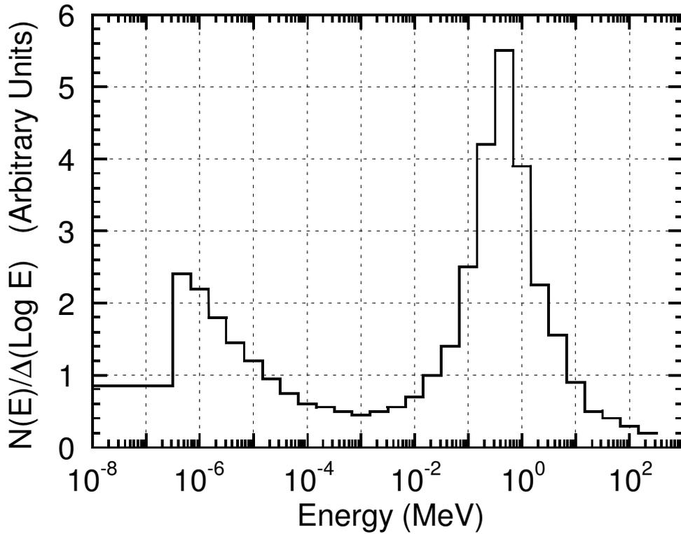
Fig. 6.6 Neutron energy spectrum (lower frame) obtained internally in a beam enclosure (upper frame) in which 800 GeV protons interacted with residual gas in the Tevatron vacuum chamber during circulating beam conditions. The site was the Fermilab Tevatron Ring. The normalization of the spectrum is arbitrary. [Adapted from (McC88).]
