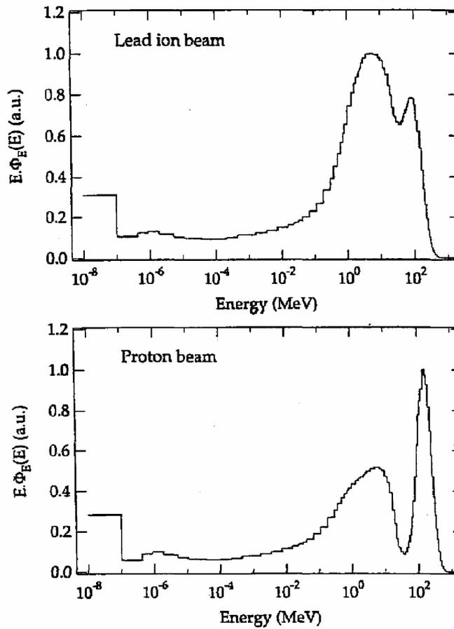
Fig. 6.11 Neutron fluence spectra around a lead ion beam of 160 GeV/nucleon shielded by concrete compared with that obtained with of a 205 GeV proton beam. The units used for the ordinate are arbitrary. For further discussion, consult the original reference of Aroua et al. [Reproduced from (Ar97).]
