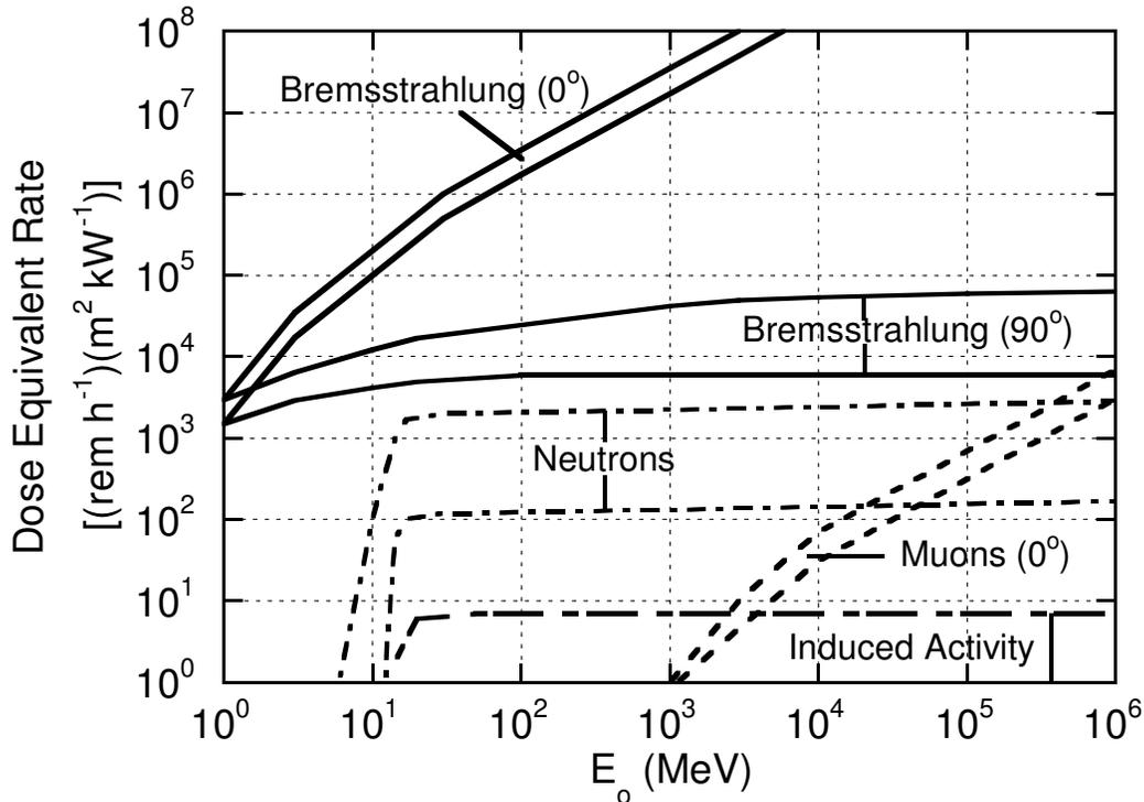
Fig. 3.10 Dose-equivalent rates per unit primary electron beam power at one meter produced by various types of "secondary" radiations from a high-Z target as a function of primary beam energy, if no shielding were present (qualitative). The width of the bands suggests the degree of variation found, depending on such factors as target material and thickness. The angles at which the various processes are most important are indicated. [Adapted from (Sw79a).]
