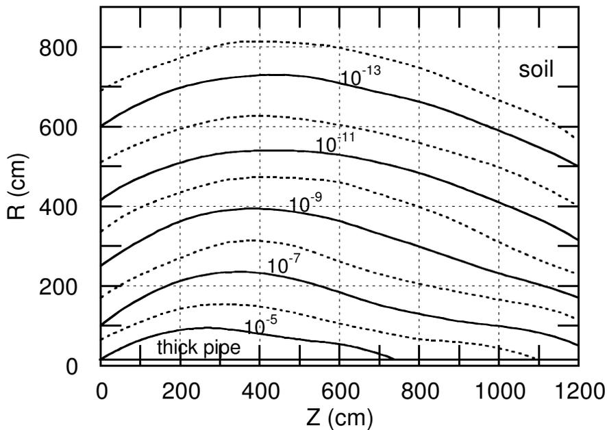
Fig. C3.d Contour plots of equal star density (stars cm<sup>-3</sup>) per incident proton calculated using CASIM for a 1 TeV proton beam incident “head on” on a thick cylindrical iron pipe of 30.48 cm outside diameter with 1.27 cm thick walls. The pipe is surrounded by soil. [Adapted from (Co82b).]
