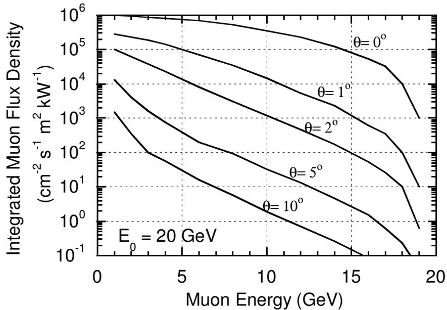
Fig. 3.9 Integrated muon flux density at 1 meter per kW of electron beam power as a function of muon energy for 20 GeV electrons incident on a thick iron target at several values of  $\theta$ . The integral of the flux density over energy includes all muons that have energies that exceed the value of the abscissa at the specified value of  $\theta$ . [Adapted from (Ne68a) and (Ne74).]
