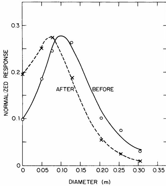
Fig. 9.5 Normalized detector response as a function of spherical moderator diameter for the situation presented in Fig. 6.8. The open circles are the measurements **before**, and the X's are the measurements **after** the placement of the additional concrete shielding. [Reproduced from (El86).]
