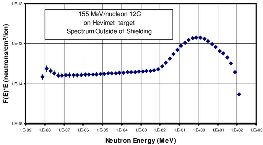
Fig. 6.10 Neutron energy spectrum  $F(E) \times E$  at 403 cm and  $\theta = 94^\circ$ , and external to 128.3 cm of concrete shielding, from a thick Hevimet target bombarded by 155 MeV/nucleon  $^{12}\text{C}$  ions [Reproduced from (Br99)].
