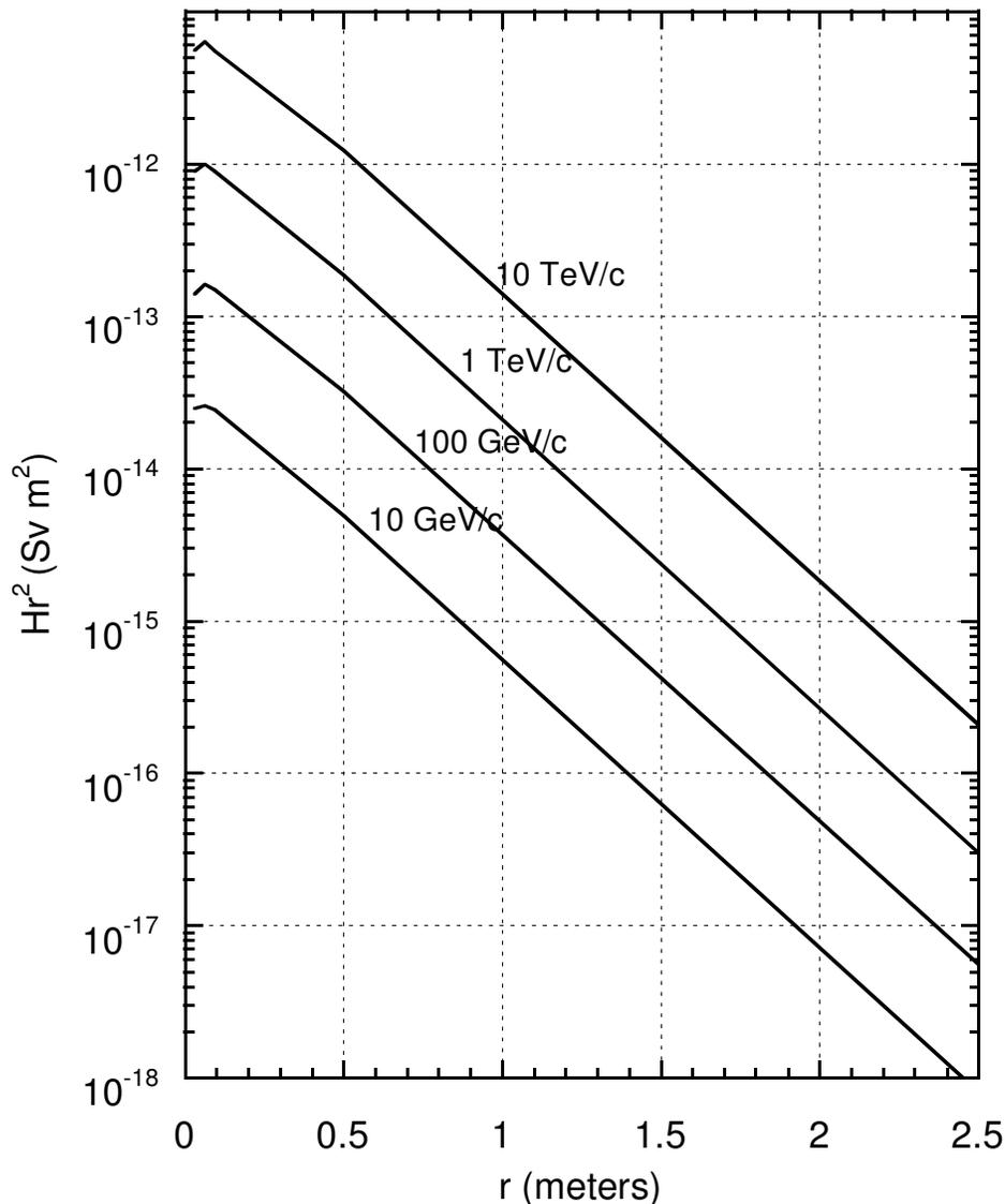
Fig. 4.24 Variation of the dose equivalent per proton at the position of the longitudinal maximum multiplied by the square of the radius,  $Hr^2$ , versus radius,  $r$ , for proton-induced cascades in IRON of density  $7.2 \text{ g cm}^{-3}$ . The coordinate  $r$  is defined as in Fig. 4.22. The results are fits to calculations obtained using FLUKA and MARS. [Adapted from (Sc90).]
