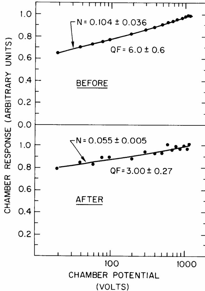
Fig. 9.17 Recombination chamber response functions measured both before (**top**) and after (**bottom**) the placement of additional shielding in the radiation field described in Fig. 6.8. [Reproduced from (E186).]
