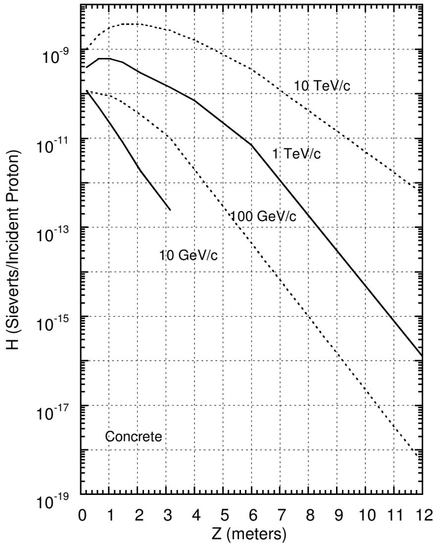
Fig. 4.26 Dose equivalent per proton,  $H$ , on the longitudinal axis,  $Z$ , as a function of depth,  $Z$ , in the shield for proton-induced cascades in CONCRETE of density  $2.4 \text{ g cm}^{-3}$ . The curves are the result of CASIM calculations for incident proton momenta of 100 GeV/c, 1 TeV/c, and 10 TeV/c and FLUKA results for 10 GeV/c. [Adapted from (Sc90).]
