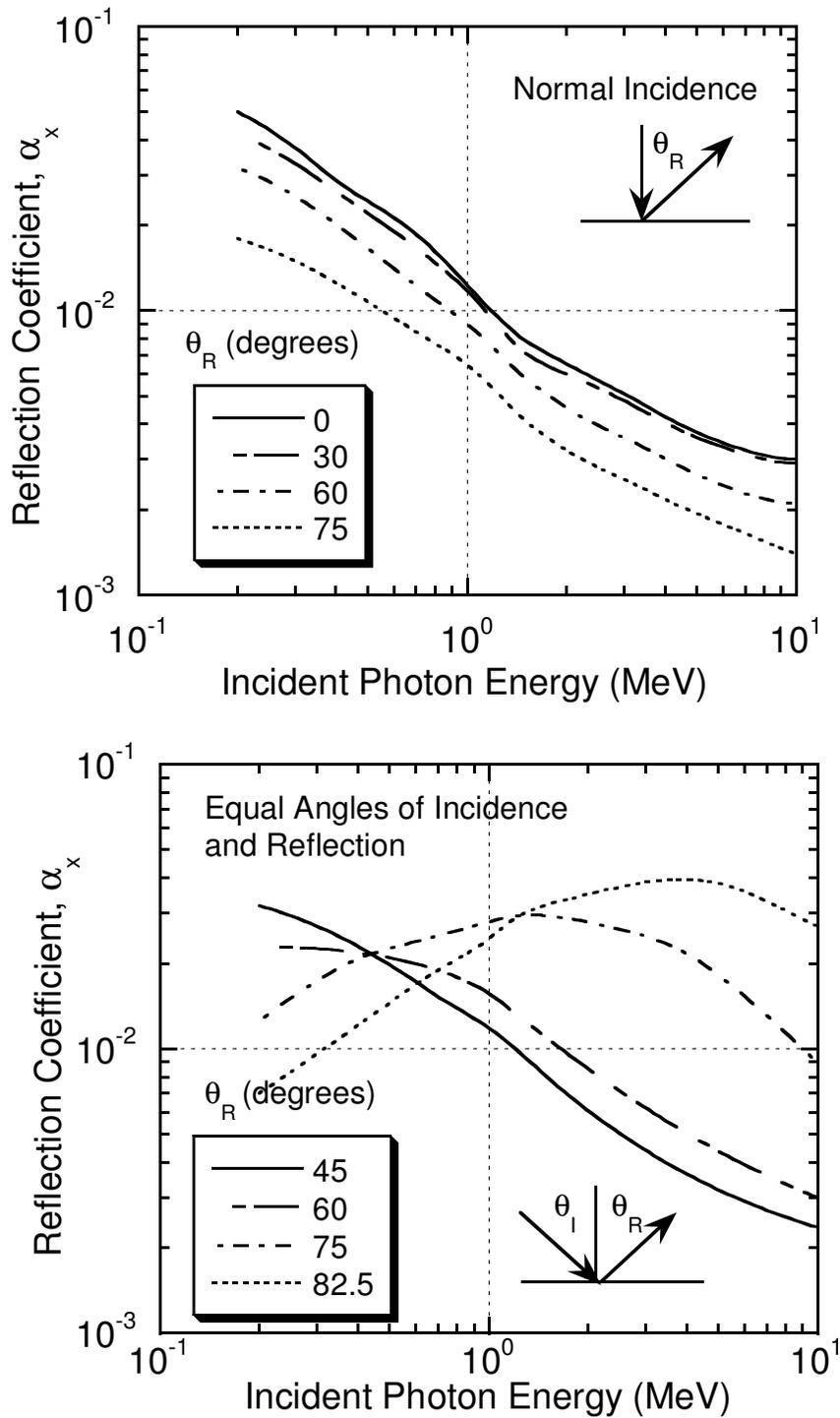
Fig. 5.1 Reflection coefficients,  $\alpha_x$ , for monoenergetic PHOTONS incident on ordinary concrete as a function of incident photon energy for several angles of reflection assuming normal incidence (**top frame**) and for equal angles of incidence and reflection ( $\theta_I = \theta_R$ ) (**bottom frame**). For photon energies higher than 10 MeV, the use of the 10 MeV values of  $\alpha_x$  is expected to be conservative. [Adapted from (NC03) and references cited therein.]
