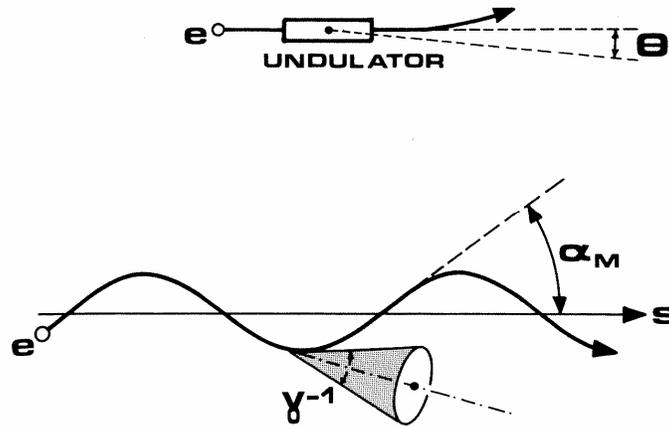
Fig. B.5 **Top:** Definition of the angle  $\theta$  at which radiation is emitted by an undulator inserted in a straight section of a storage ring. **Bottom:** Angular amplitude of the half-angle of the cone of emission of radiation,  $\approx \gamma^{-1}$ , and maximum deflection angle of the electron trajectory caused by an insertion device,  $\alpha_m$ . [Adapted from (Ma88).]
