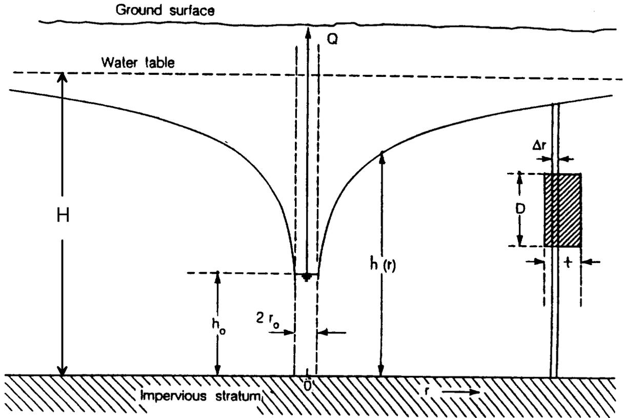
Fig. 8.6 Hydrogeological model of a shallow well in proximity to an accelerator tunnel where a beam loss occurs. The radioactivated region is represented in cross section by the cross-hatched rectangle to the right.  $h$  represents the elevation of the water table above the impervious stratum as a function of  $r$  while the water table is a distance  $H$  above the impervious stratum where the water table is not perturbed by wells. [Adapted from (Ja87).]
