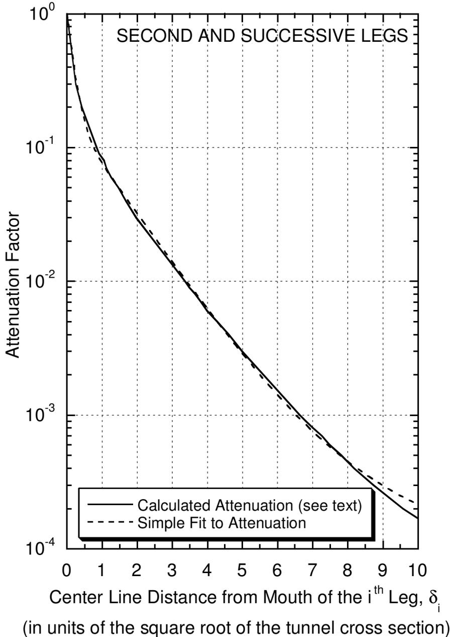
Fig. 5.8 Universal transmission curve for the second and subsequent legs of labyrinths as a function of normalized distance from the center of the previous turn,  $\delta_i$ . The calculated attenuation (solid curve) is the calculation made using AMC by Goebel et al. (Go75). The dashed curve is the fit provided by Eq. (5.7). [Adapted from (Go75) and (Co95).]
