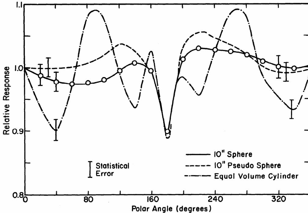
Fig. 9.9 Relative neutron detection efficiency of three different moderators with a 4 x 4 mm<sup>2</sup> cylindrical <sup>6</sup>LiI(Eu) detector at the center. The efficiencies are plotted as a function of the polar angle. The polar angle is measured from the axis of the light pipe. [Adapted from (Aw72).]
