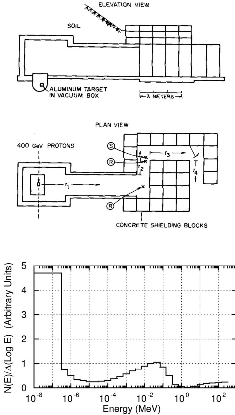
Fig. 6.7 Neutron energy spectrum (**lower frame**) obtained within a labyrinth enclosure (**upper frame**) in which 400 GeV protons interacted with an aluminum target located beneath the floor of the enclosure shown. The spectrum was measured in the second leg at the location denoted "S". A quality factor measurement was made at the locations denoted "R" (see Sections 5.2.4 and 9.5.7). The normalization of the spectrum is arbitrary. [Adapted from (Co88).]
