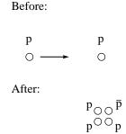
In this scenario the kinetic energy of the incoming projectile is completely converted into the rest energy of the created proton and antiproton. Hence at threshold the incoming projectile would need kinetic energy  $2m_{\rm p}c^2$  or total energy  $3m_{\rm p}c^2$ .
