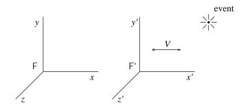
Suppose an event happens. That event has space-time coordinates (x, y, z, t) in inertial frame F and space-time coordinates (x', y', z', t') in inertial frame F'. If frame F' moves at constant speed V relative to frame F, and the two frames coincide at time t = t' = 0, then we know that the two sets of coordinates are related through the Lorentz transformation:
