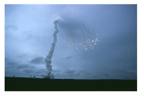
In 1996, a European Ariane 5 rocket was set to deliver a payload of satellites into Earth orbit, but problems with the software caused the launch rocket to veer off its path a mere 37 seconds after launch. The problem was the result of code reuse from the launch system's predecessor, Ariane 4, which had very different flight conditions from Ariane 5.
